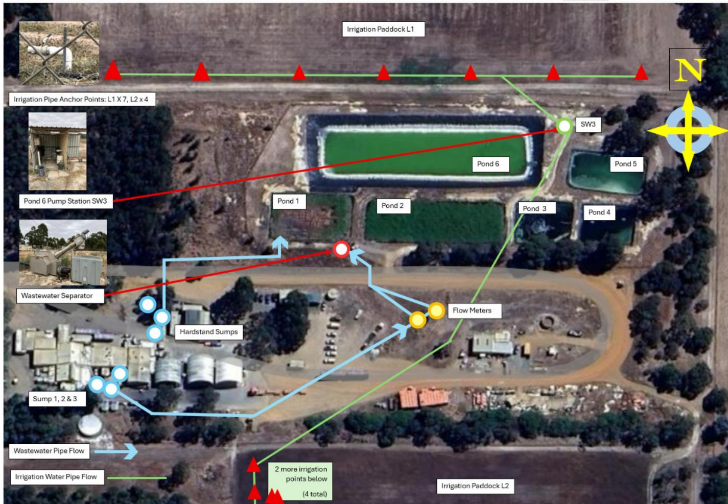
Figure 3: Wastewater delivery plan
