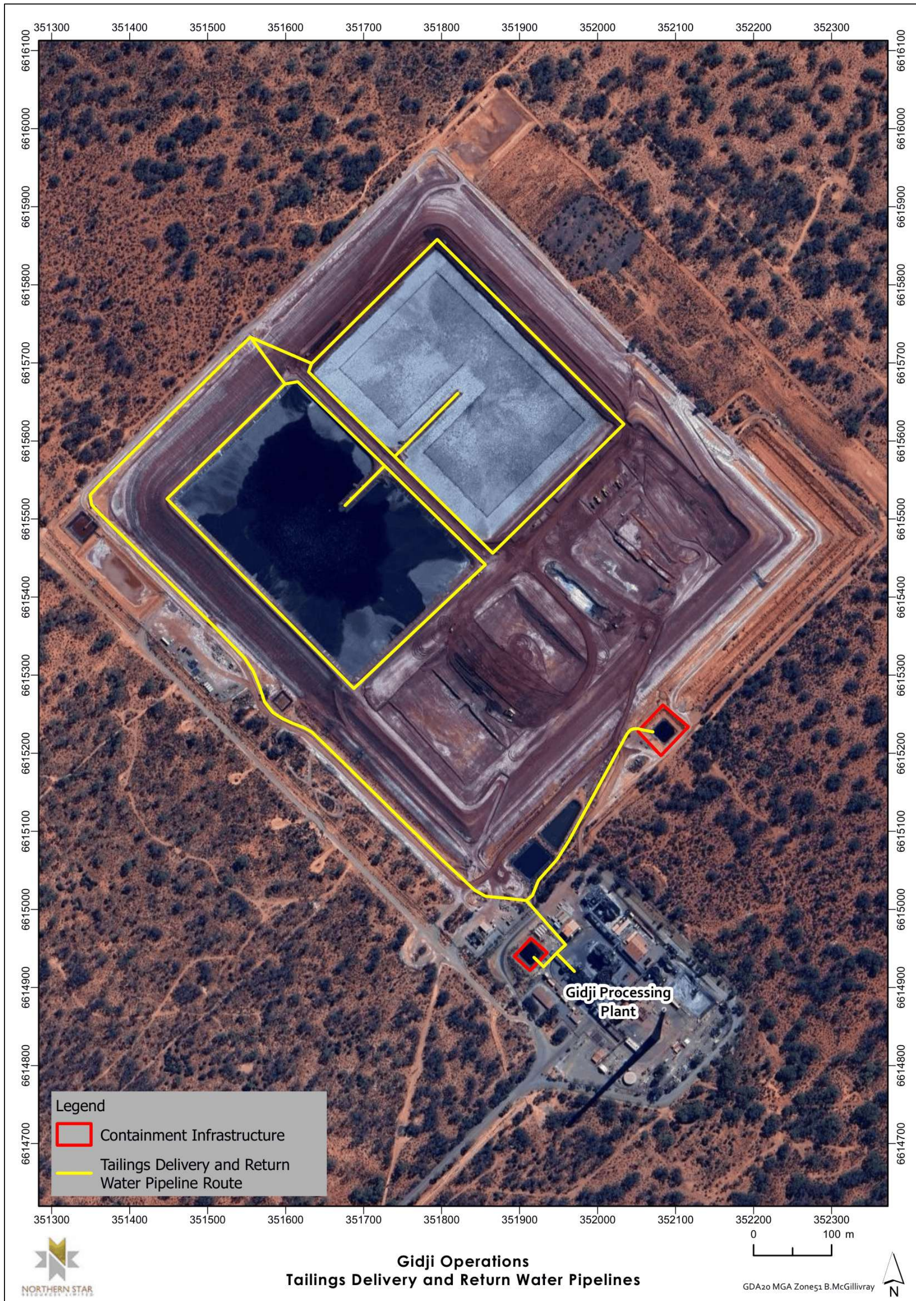
Figure 3: Tailings delivery and return water pipelines
