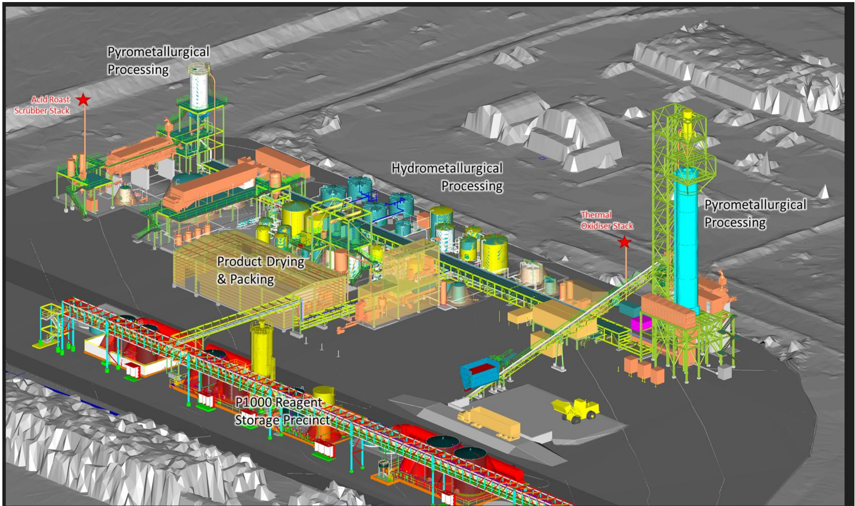
Figure 13: Mid-Stream Demonstration Plant Site Plan
