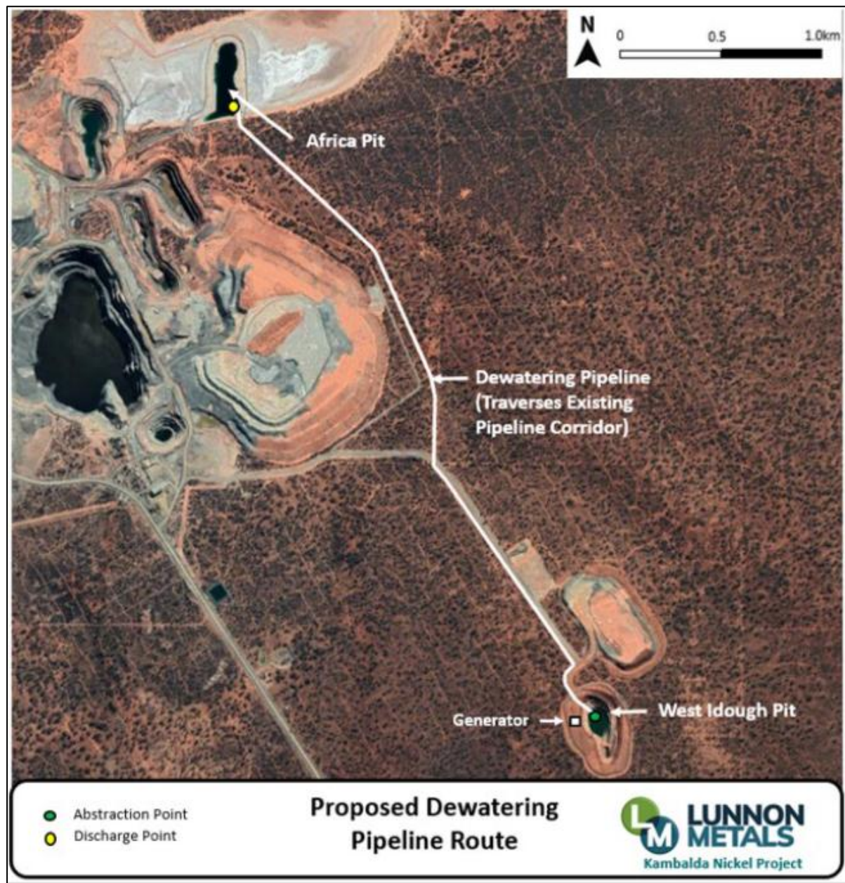
Figure 2: Map of the dewatering pipeline, generator, abstraction and discharge locations.
