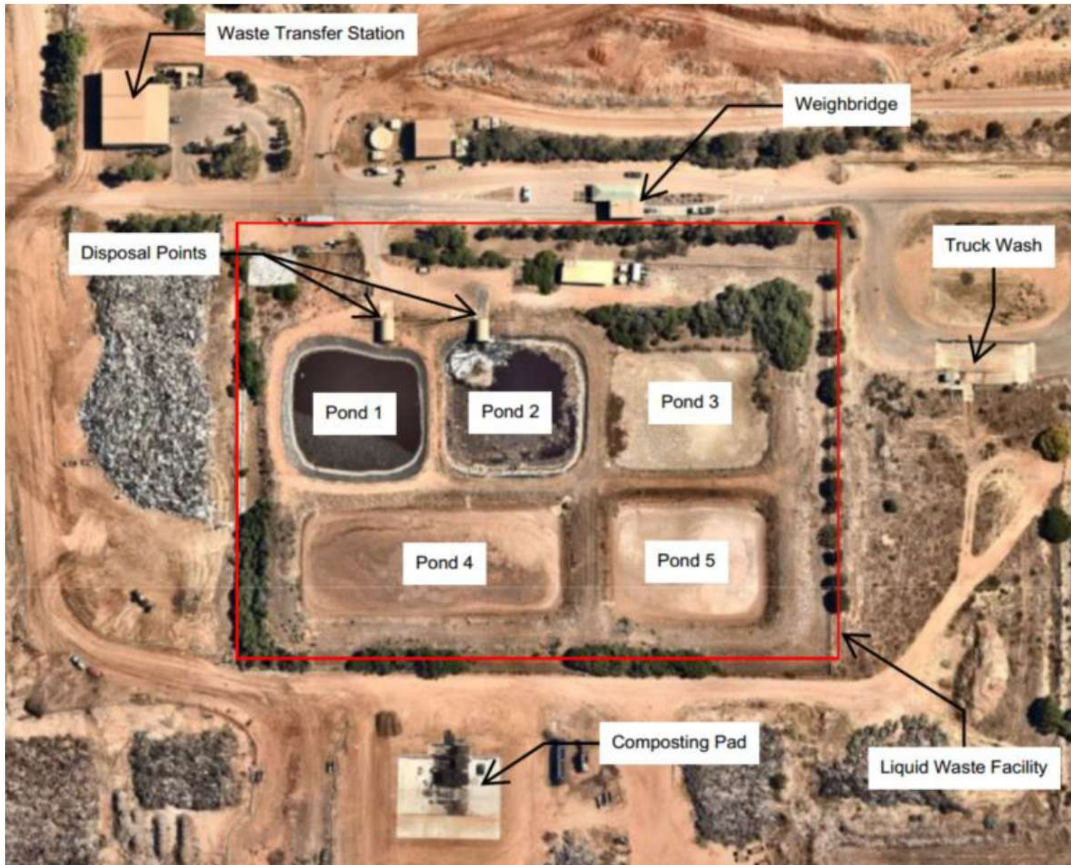
Figure 5: Liquid Waste Facility Layout
