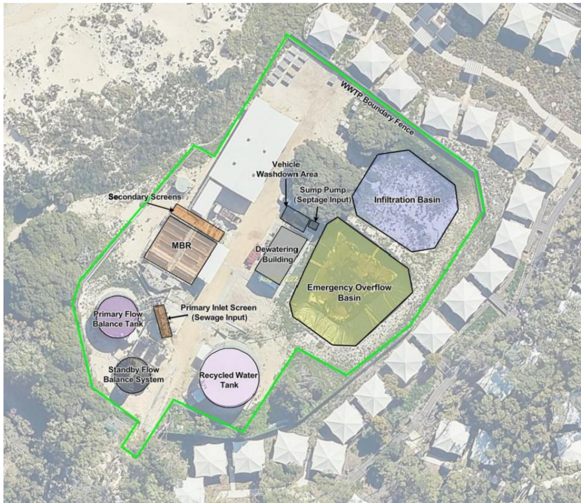
Figure 2: WWTP site plan
