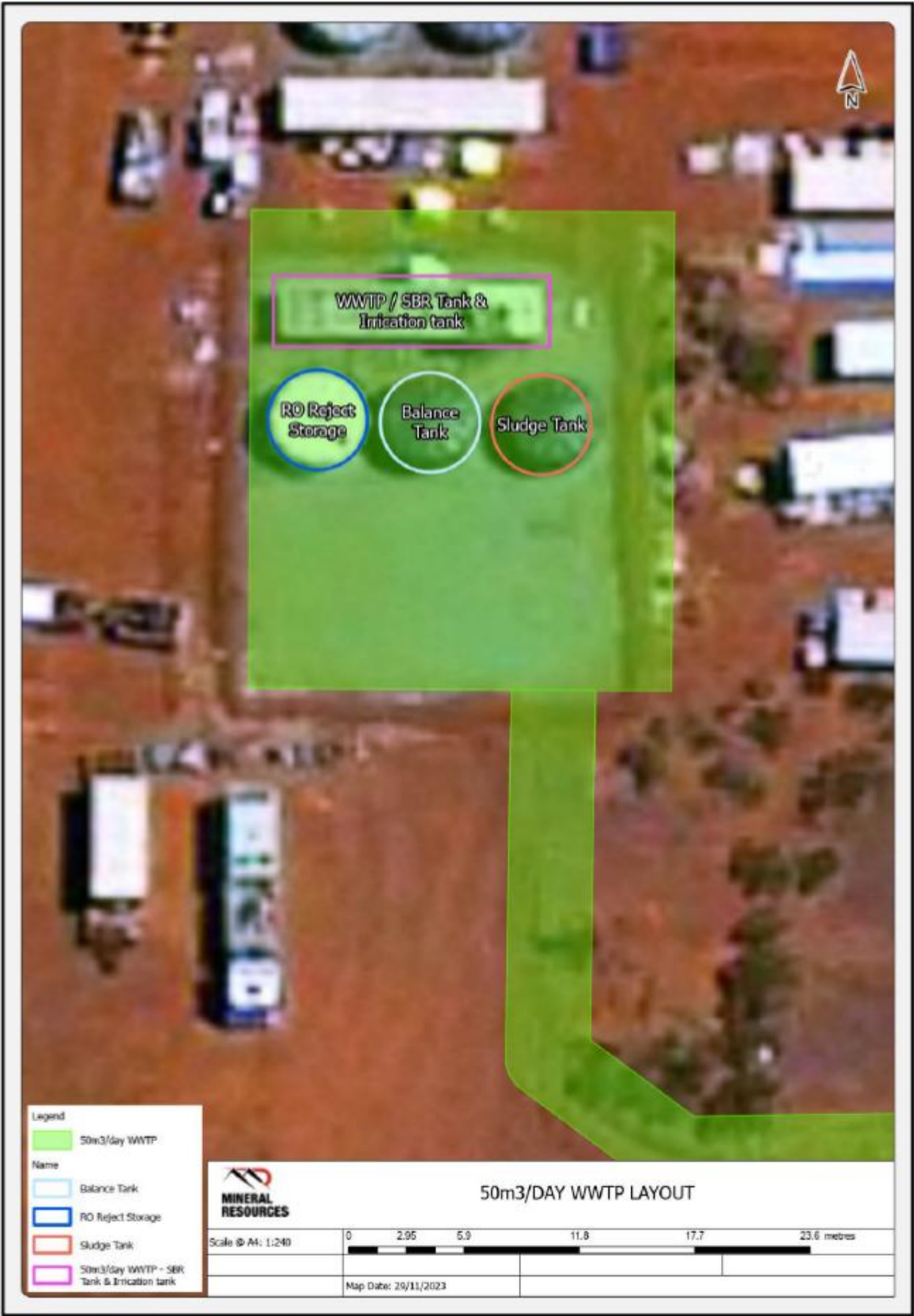
Figure 7: Layout of Construction Camp WWTP (50 m³/day)
