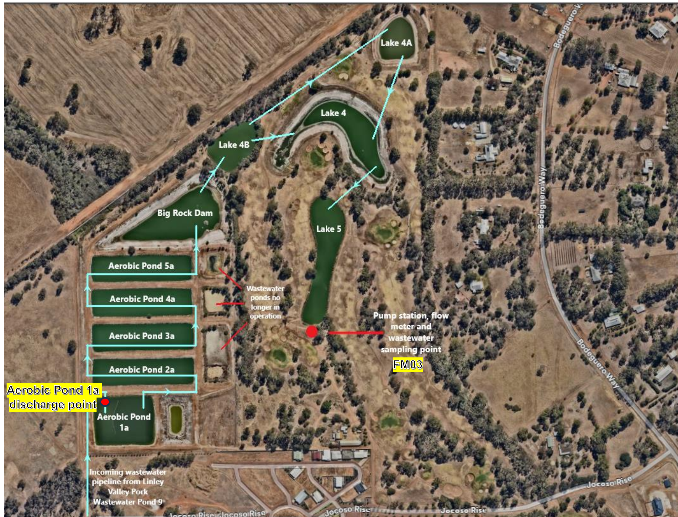
Figure 8: Map of the secondary wastewater treatment system - storage ponds and lakes layout and flow direction
