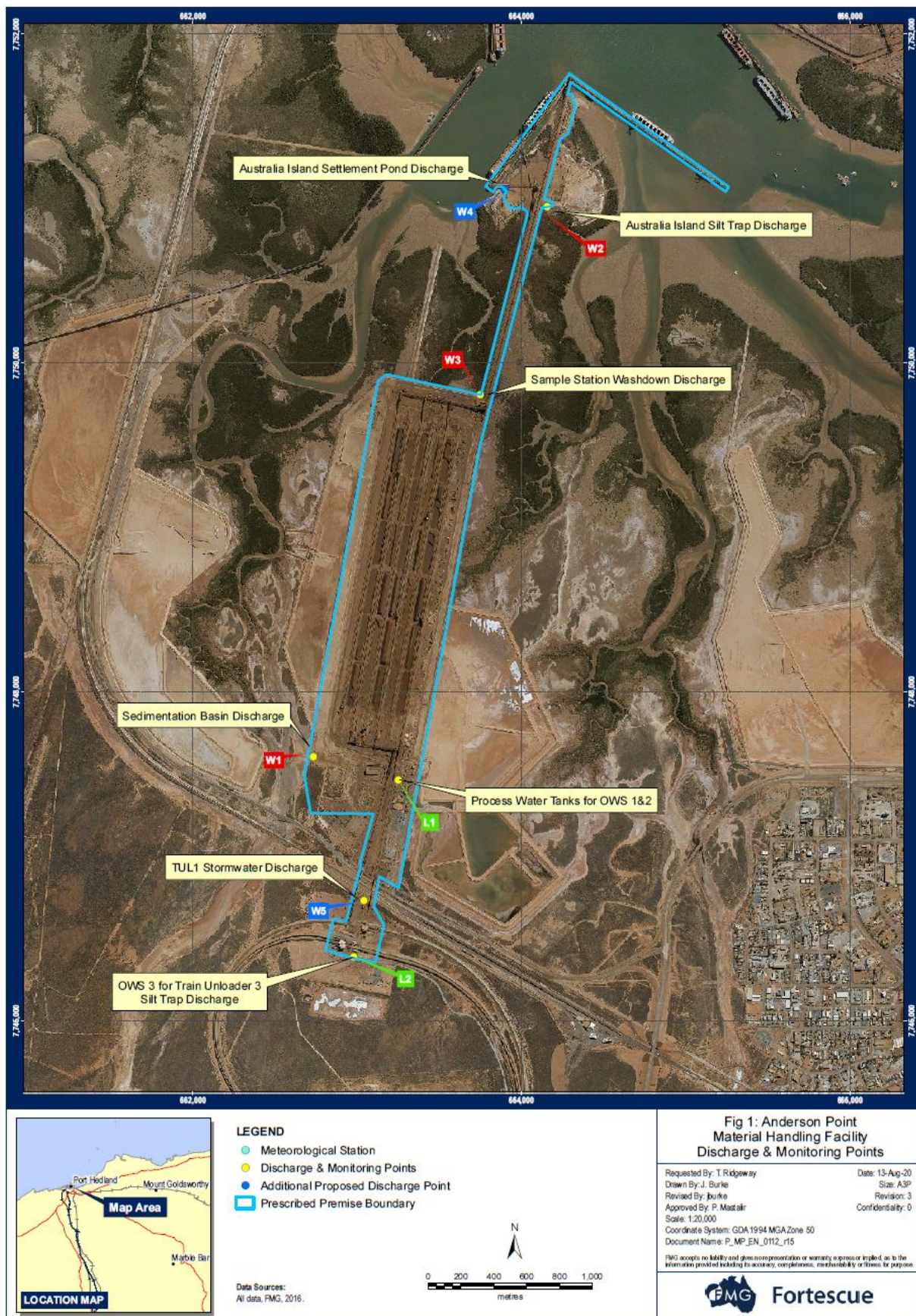
Figure 9: Stormwater and washwater discharges
