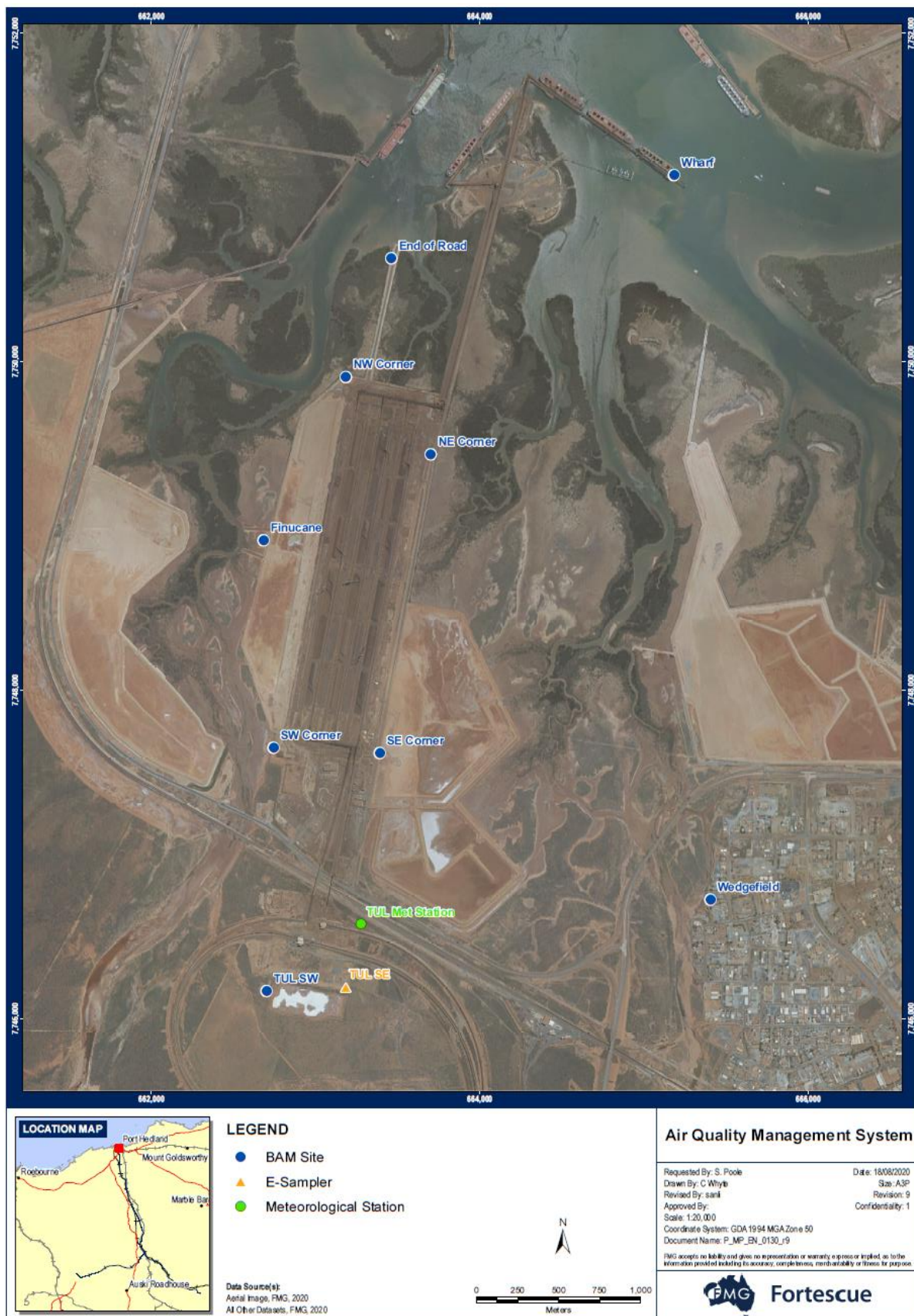
Figure 6: Premises dust monitoring network
