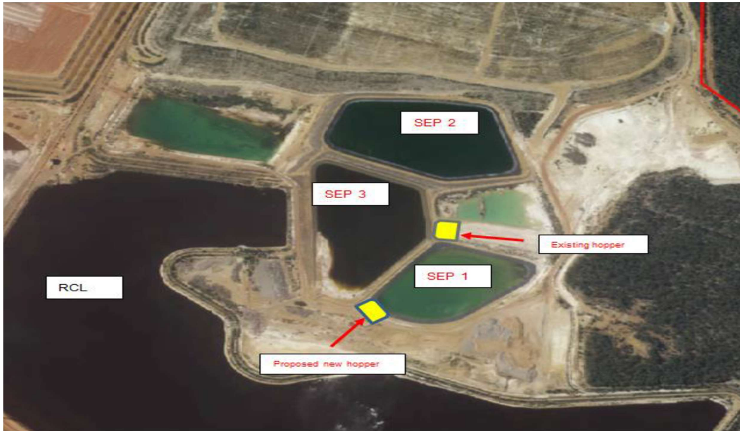
Figure 1: Map for the location of the new SEP1 hopper in relation to Solar Evaporation Pond 1 (SEP1) and the Refinery Catchment Lake (RCL)
