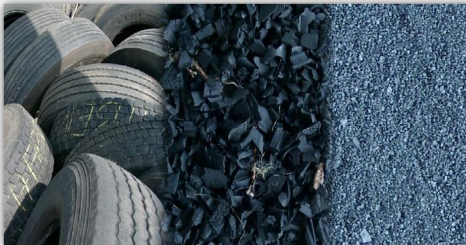
Fig. 11 Raw material (whole tyres), tyre shred, and tyre crumb
