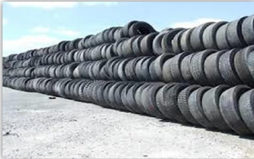
Fig. 6.2.1 “Tread up” Storage with Inadequate Separation Gaps
