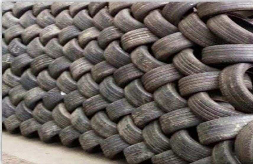
Fig. 6.1.4 Tyres Stacked in Laced Arrangement - Outdoor Storage Only
