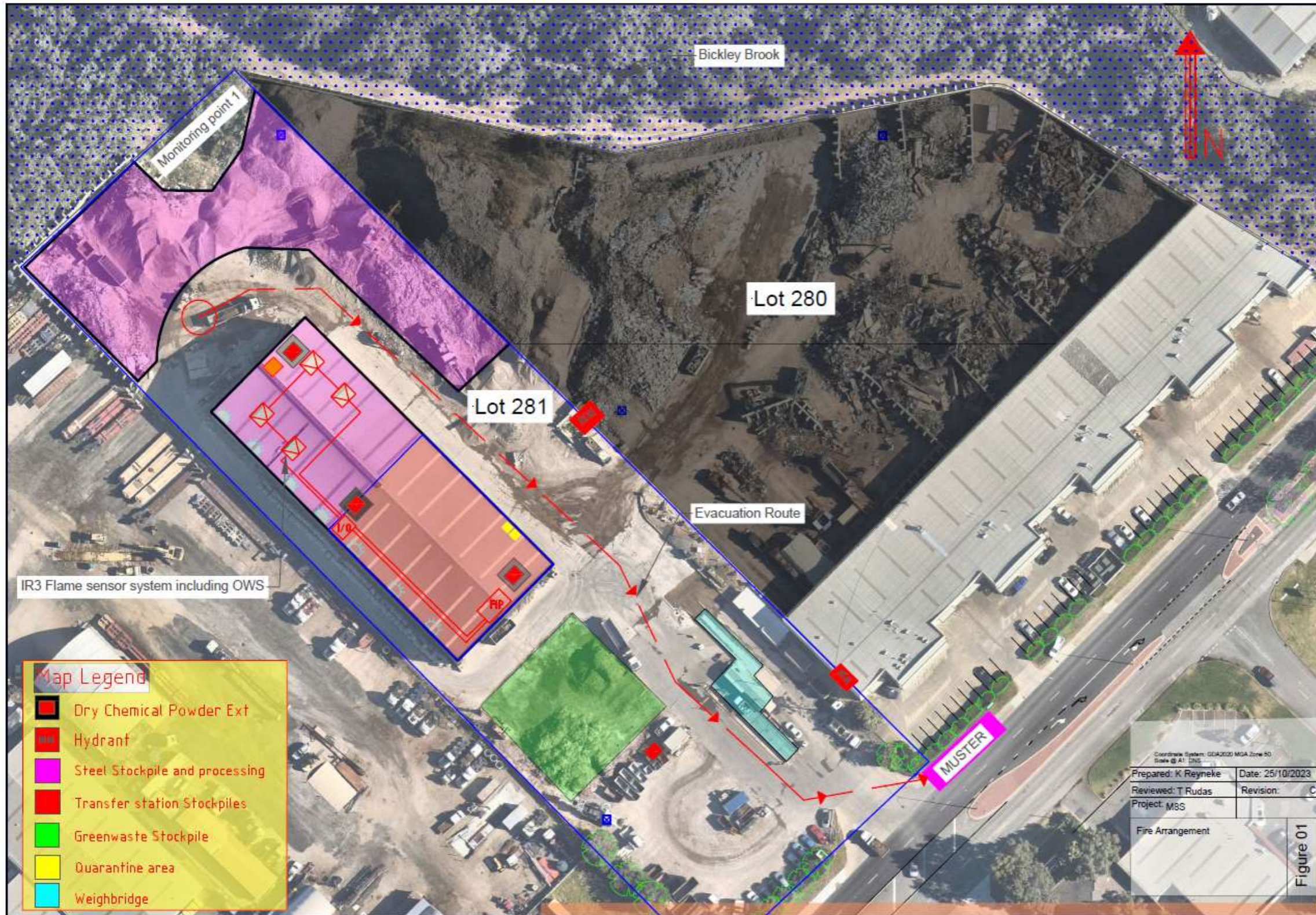
Figure 3: Fire and Emergency Arrangement
