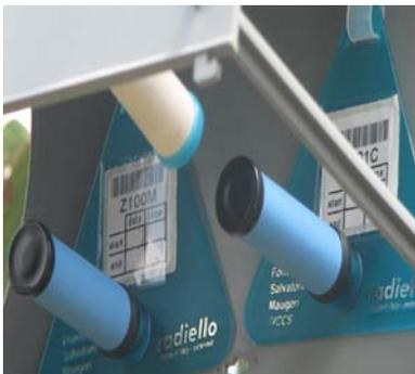
Figure 2: Passive samplers
