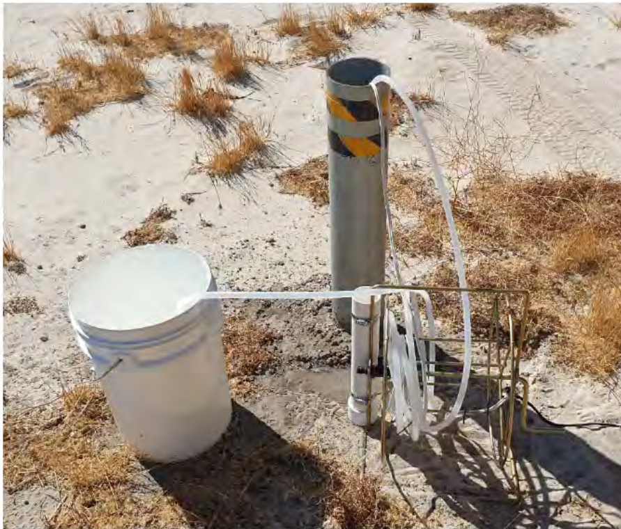
Photograph 4: Pump lowered into bore and discharge hose directed to bucket.
