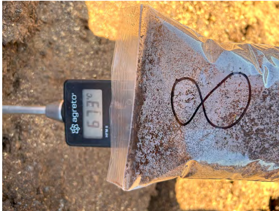
Photograph 12 – KDFP – Monitoring equipment – Manure/Compost Temperature Probe
