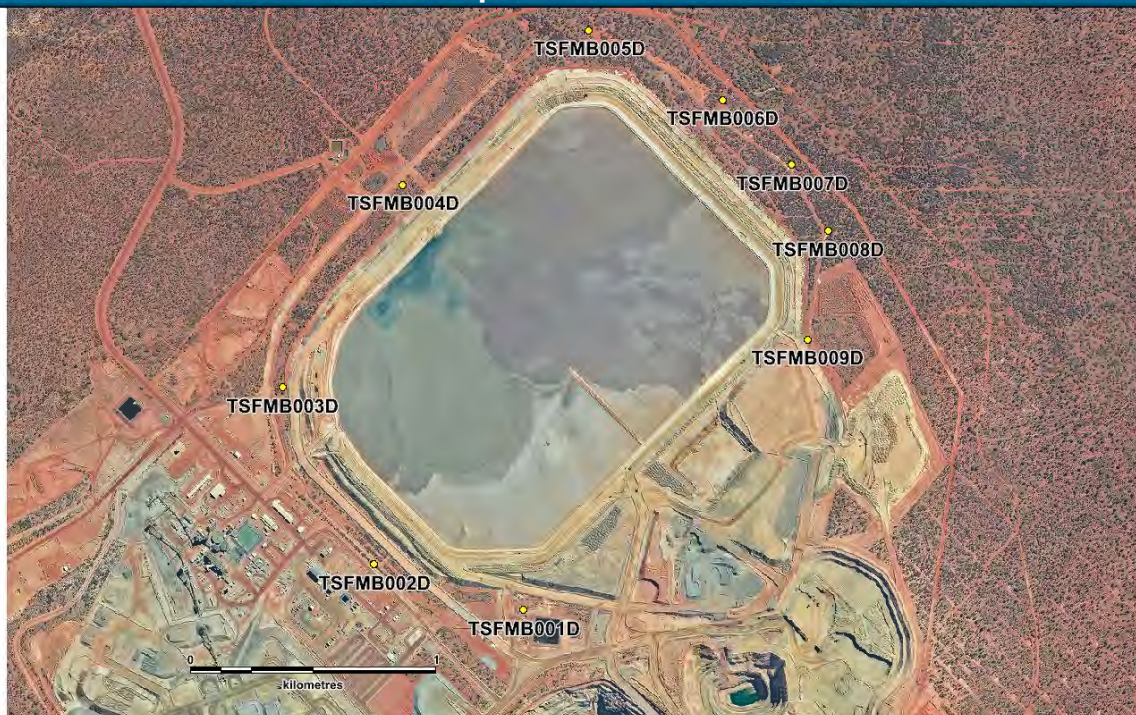
Figure 3 – TSF Monitoring Bore Locations
