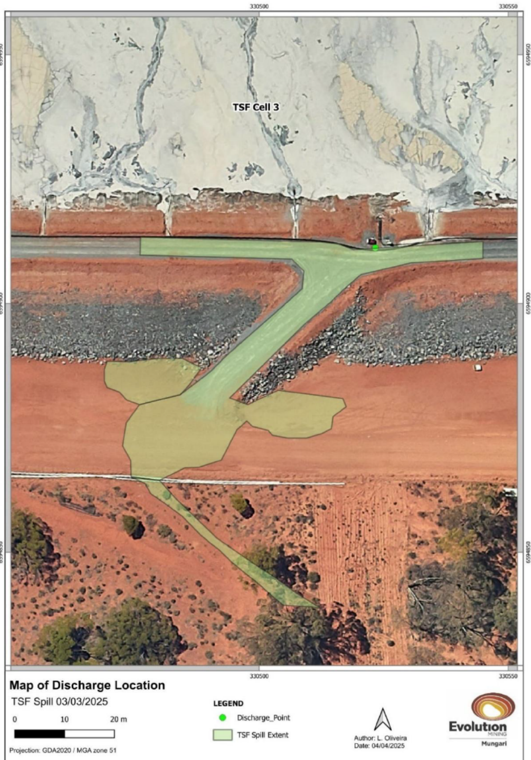
Figure 2: TSF Spigot Failure Location
