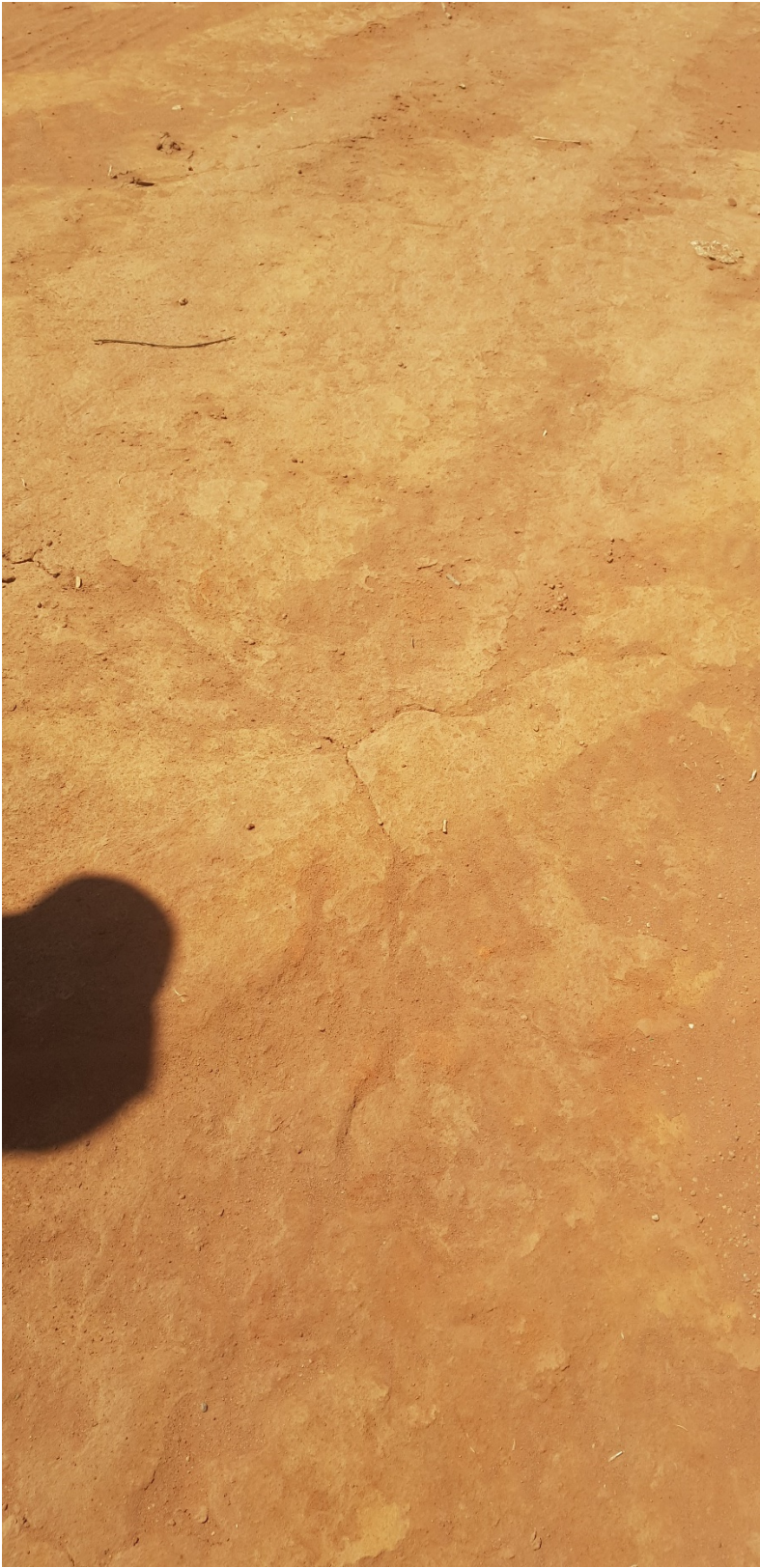
Figure 5. This picture shows the type of clay that lines the bottom of the liquid waste ponds. The clay dries very hard.
