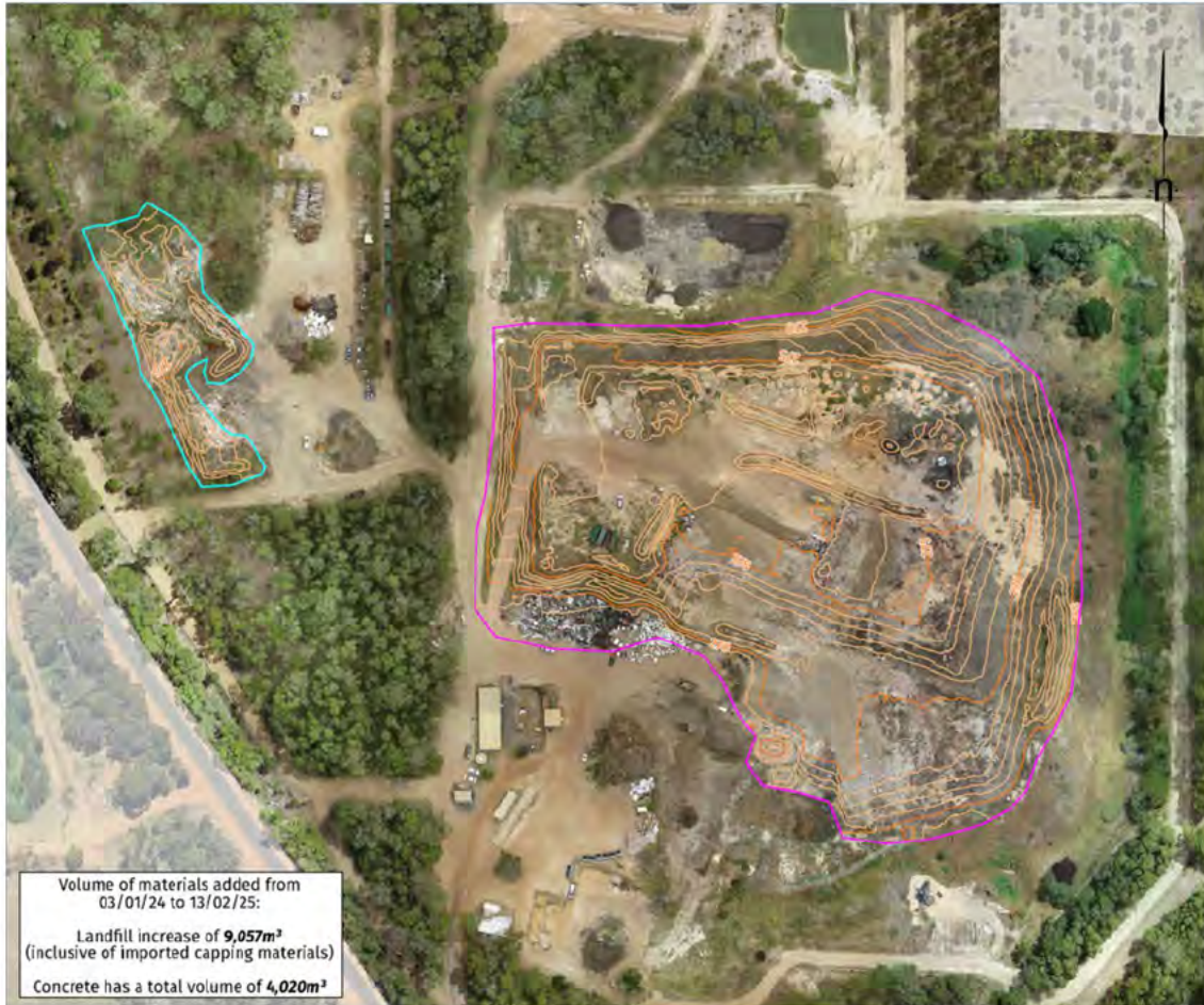
Figure 3: Drone image generated by Harley Dykstra for the volumetric survey carried out on 13/02/2025. (Larger image attached as Attachment 4 of BER)
