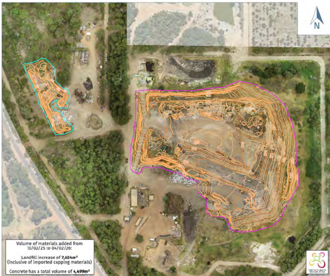
Figure 4: Drone image generated by Harley Dykstra for the volumetric survey carried out on 04/02/2026. (Larger image attached as Attachment 4 of BER)
