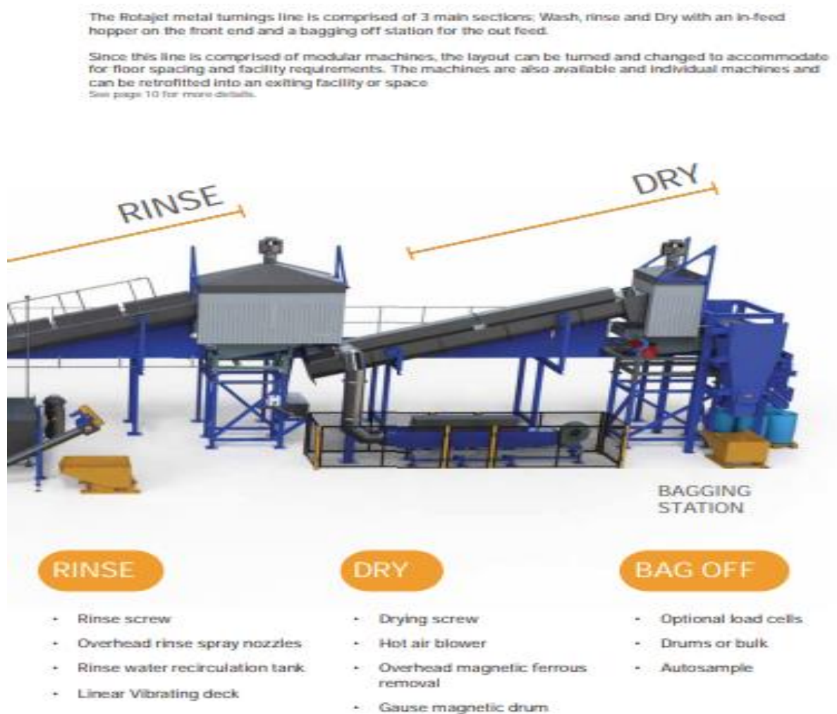
Figure 1: Basic structure of the rotajet swarf washing line
