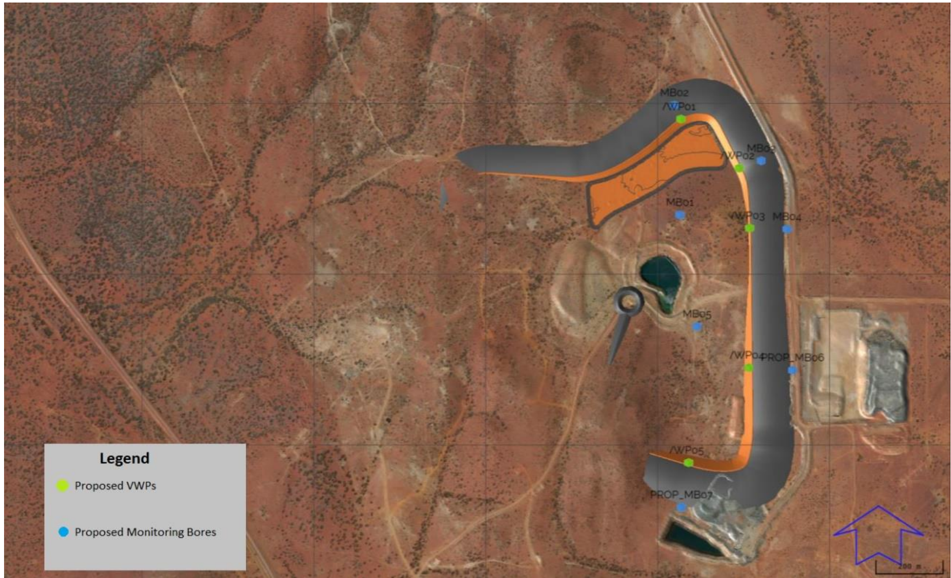
Figure 8: Monitoring infrastructure for IWL TSF (Stage 1-3)
