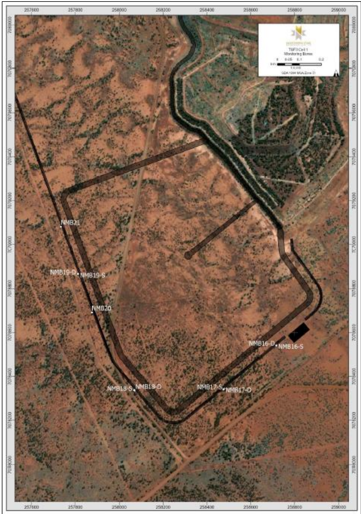
Figure 2: Installed groundwater monitoring bores around TSF 3 cell 1. D and S indicate a deep and shallow bore respectively.
