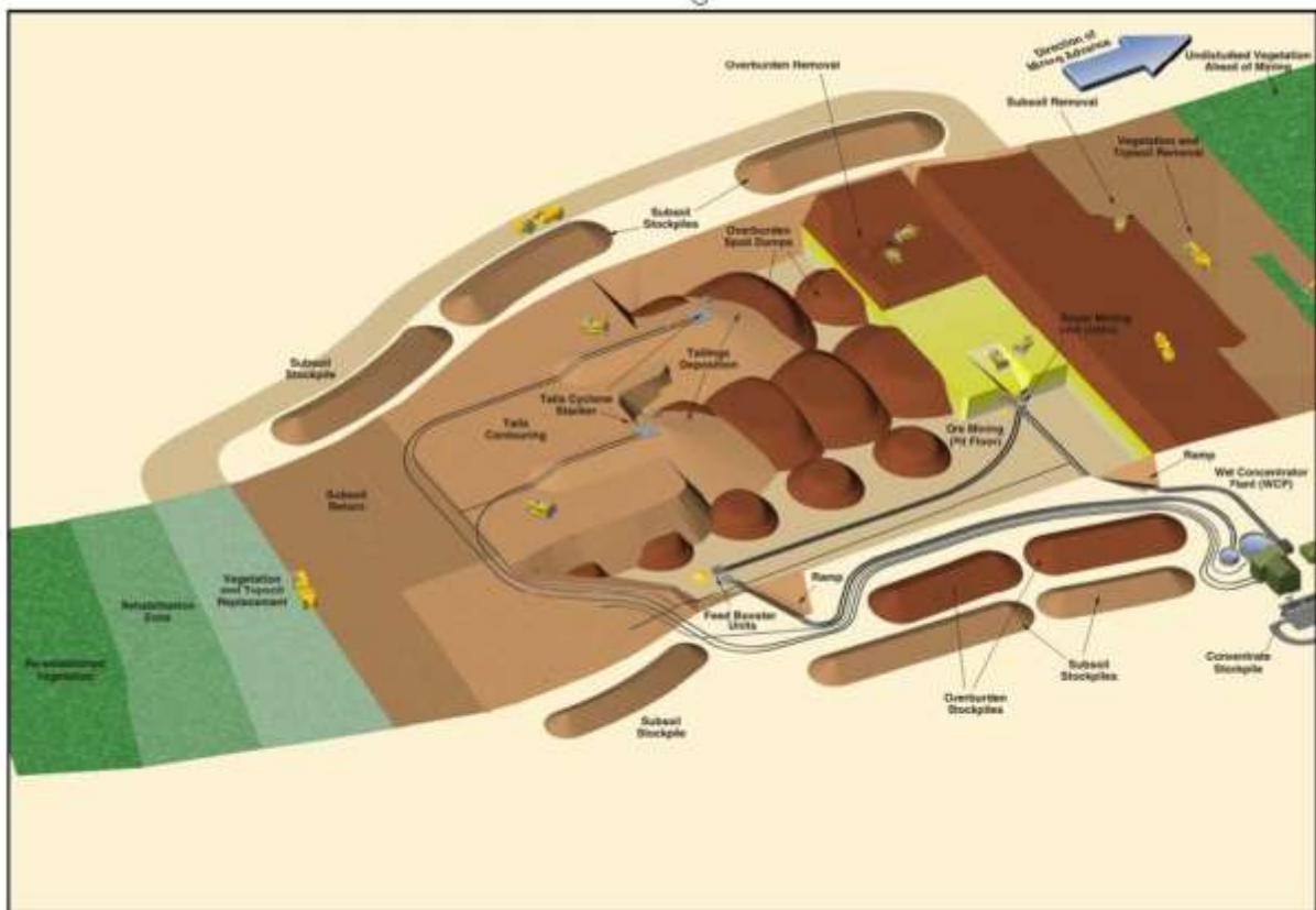
Figure 2: Conceptual layout of mining operations
