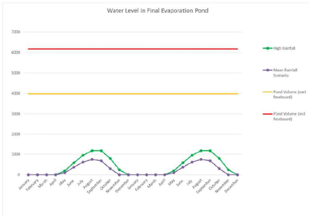
Figure 3: Water balance model showing water level in the final evaporation pond in kilolitres
