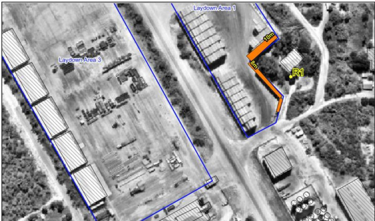
Figure 4: Designated barriers (4 or 5 retainers high) for noise mitigation at night to R1
