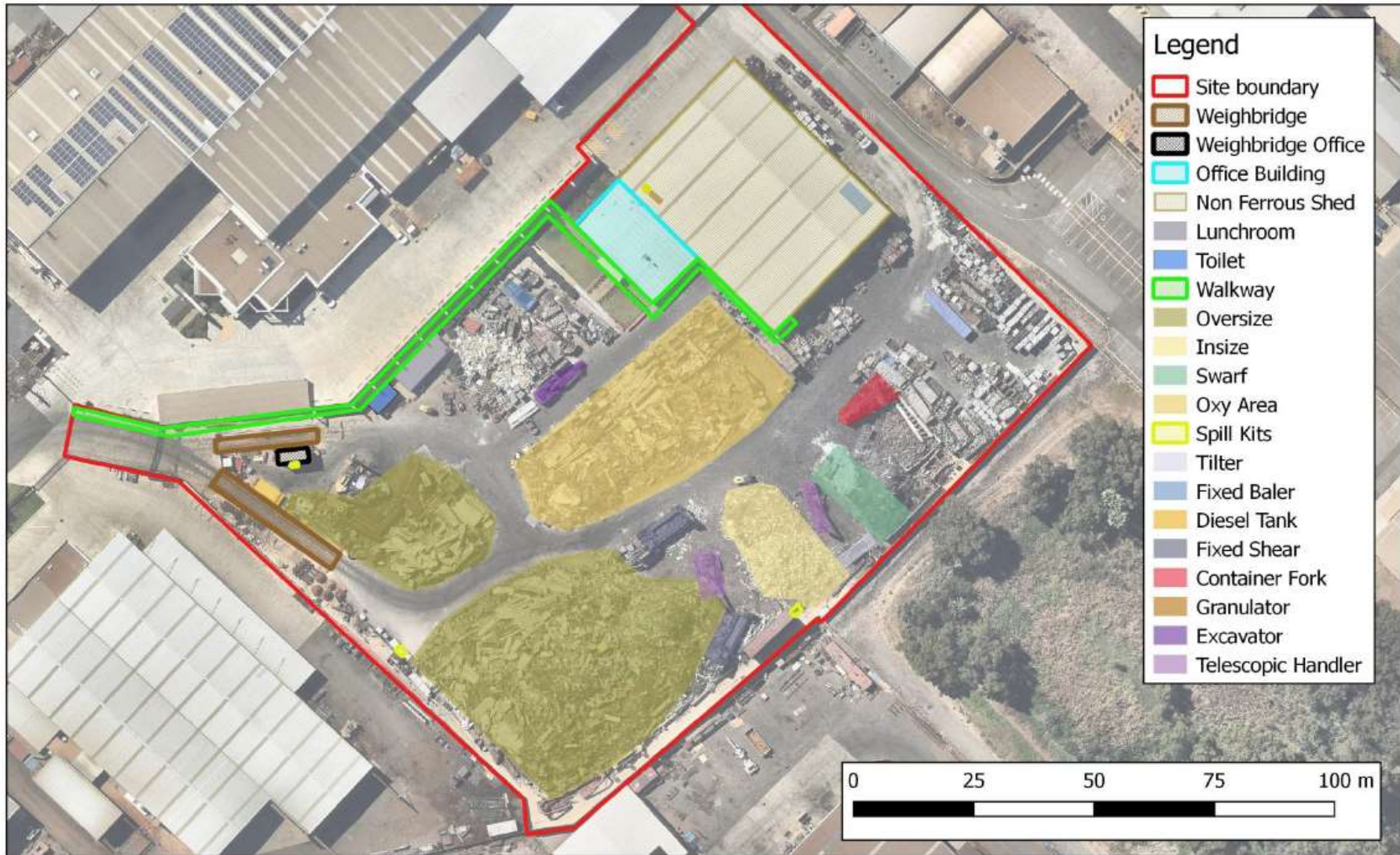
Figure 1: Aerial overview of Premises
