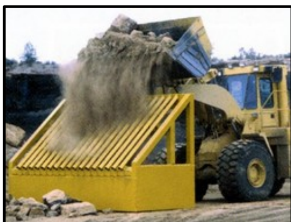
Figure 1: Photos of the Grizzly screen in operation
