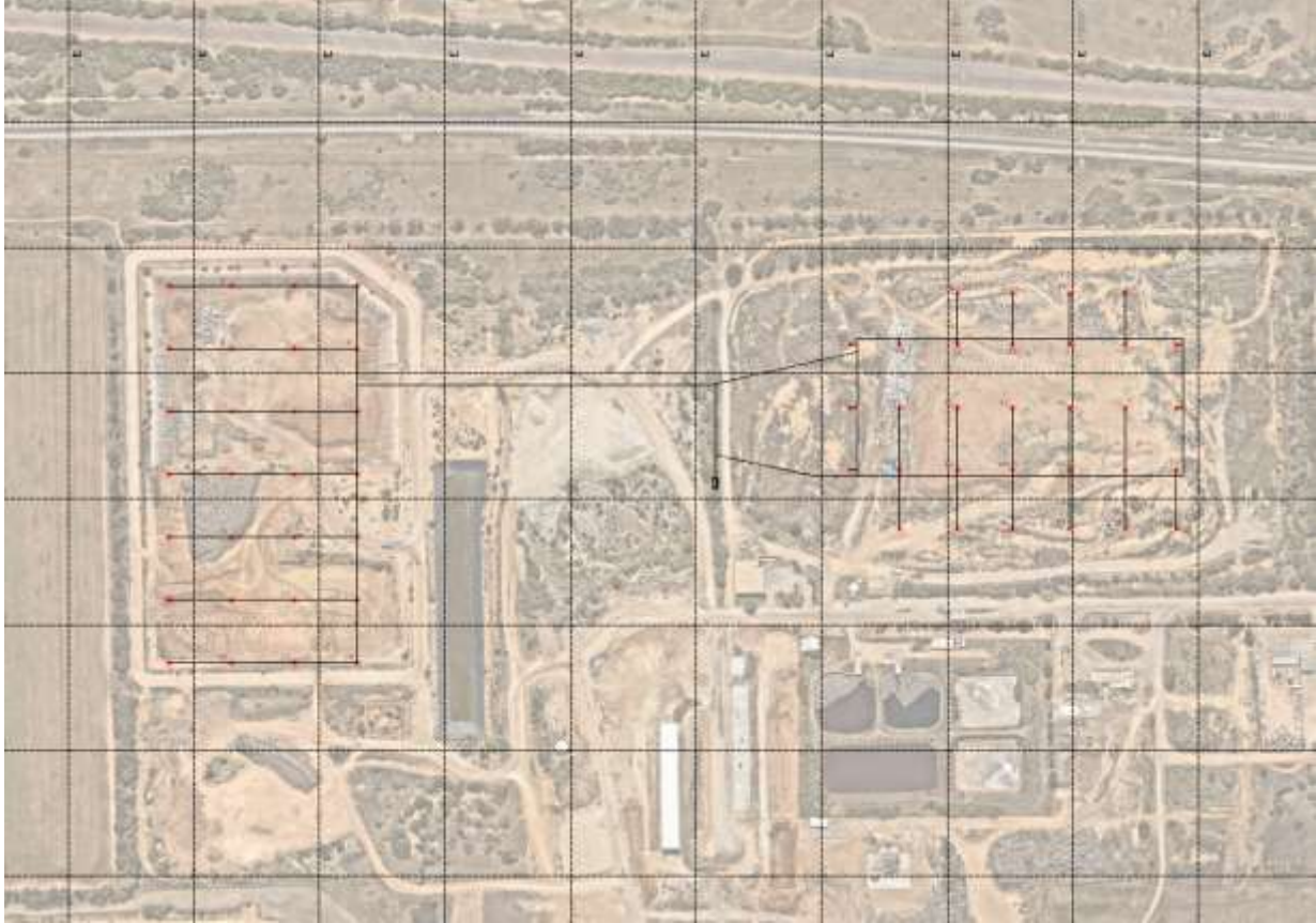
Figure 1: Proposed landfill gas extraction wells
