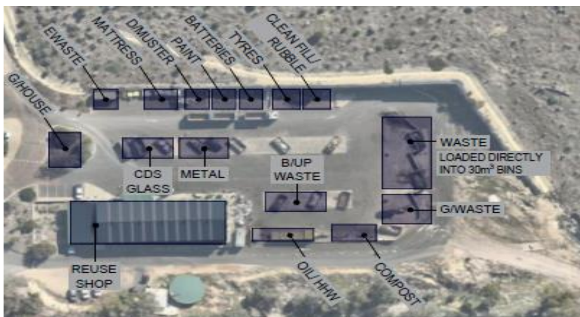
Figure 2: Layout of the transfer station
