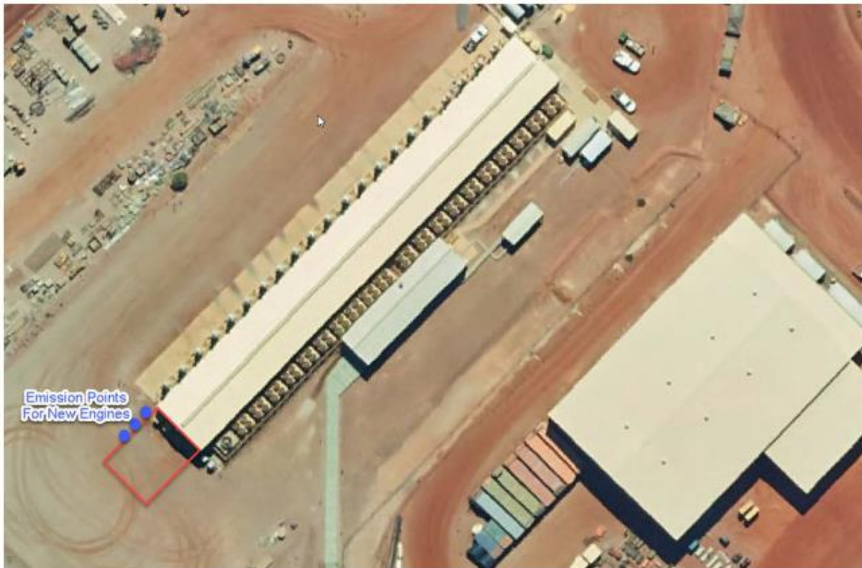
Figure 2: Approximate location of emission points for the proposed new power station generators
