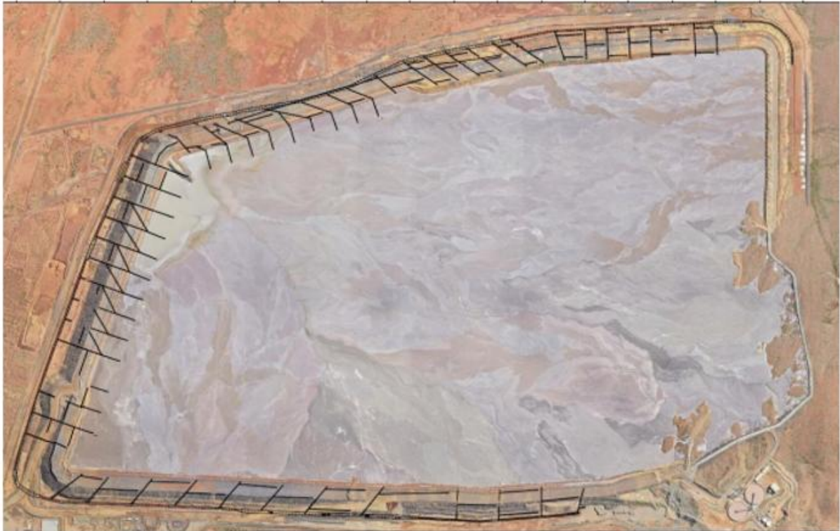
Figure 2: Finger Drains Layout below the TSF2 embankments
