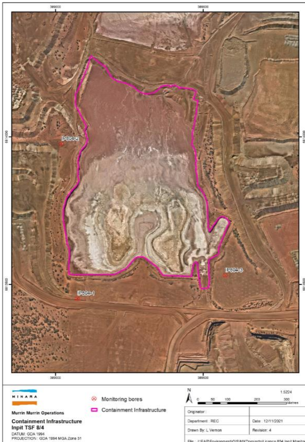
Figure 2: 8/4 in-pit TFS and related monitoring bores.
