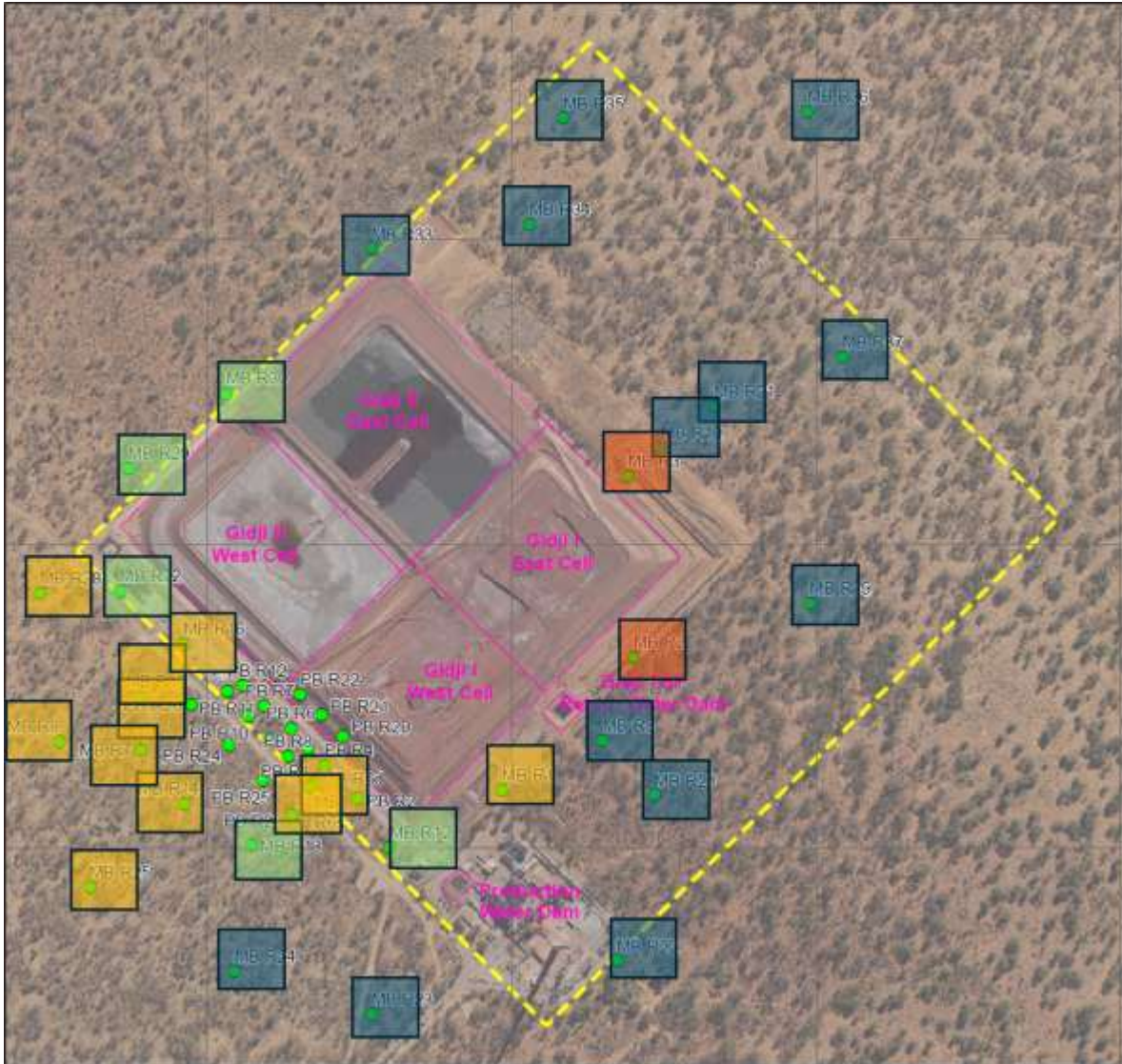
Figure 7: Groundwater level at the premises, represented by blue boxes (approx. 20 mbgl or deeper), green boxes (between 10 to 20 mbgl), yellow boxes (10 mbgl or shallower), and orange boxes (10 mbgl or shallower, with at least one exceedance of 6 mbgl between 2022 and 2025)
