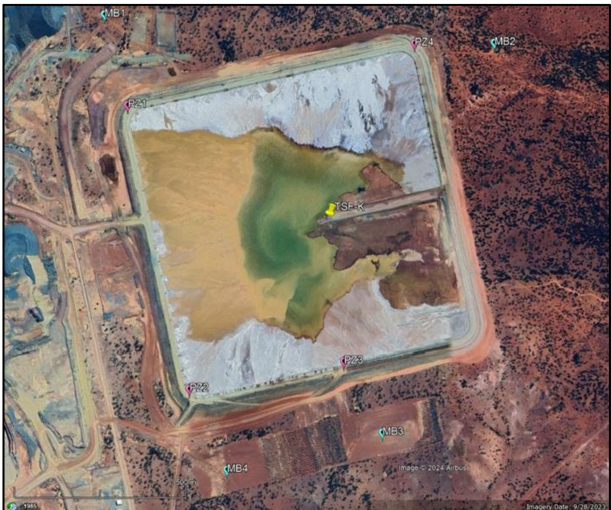
Figure 5. Location of current groundwater bores (MB1-4, equivalent to TD17K-20K on the licence) and standpipe piezometers (PZ1-4)
