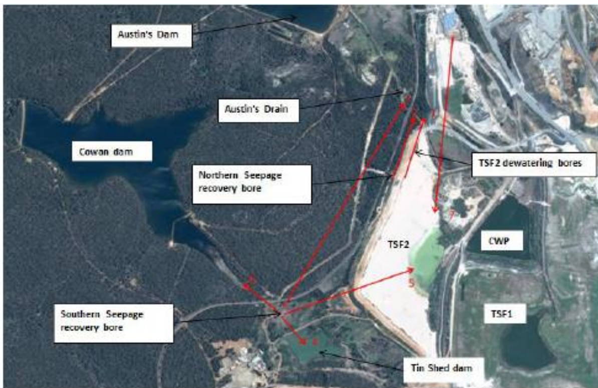
Figure 10: Current TSF2 drainage management plan
