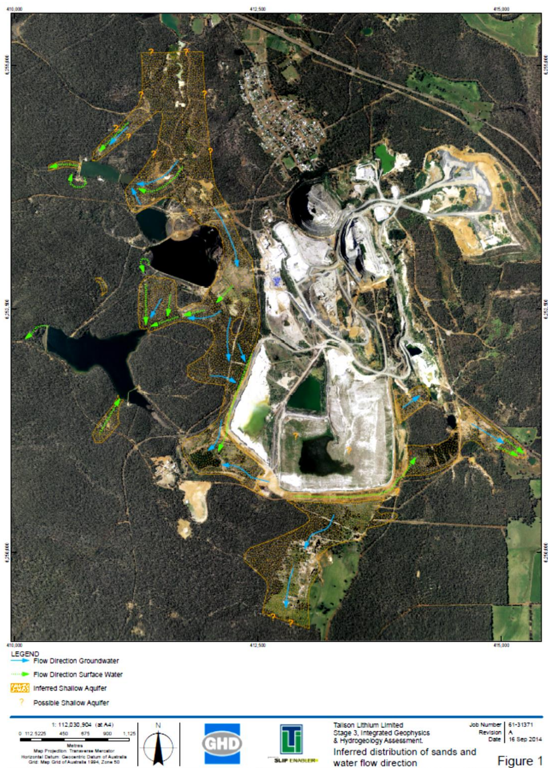
Figure 9: Inferred shallow aquifer flow direction and distribution (GHD 2014b)
