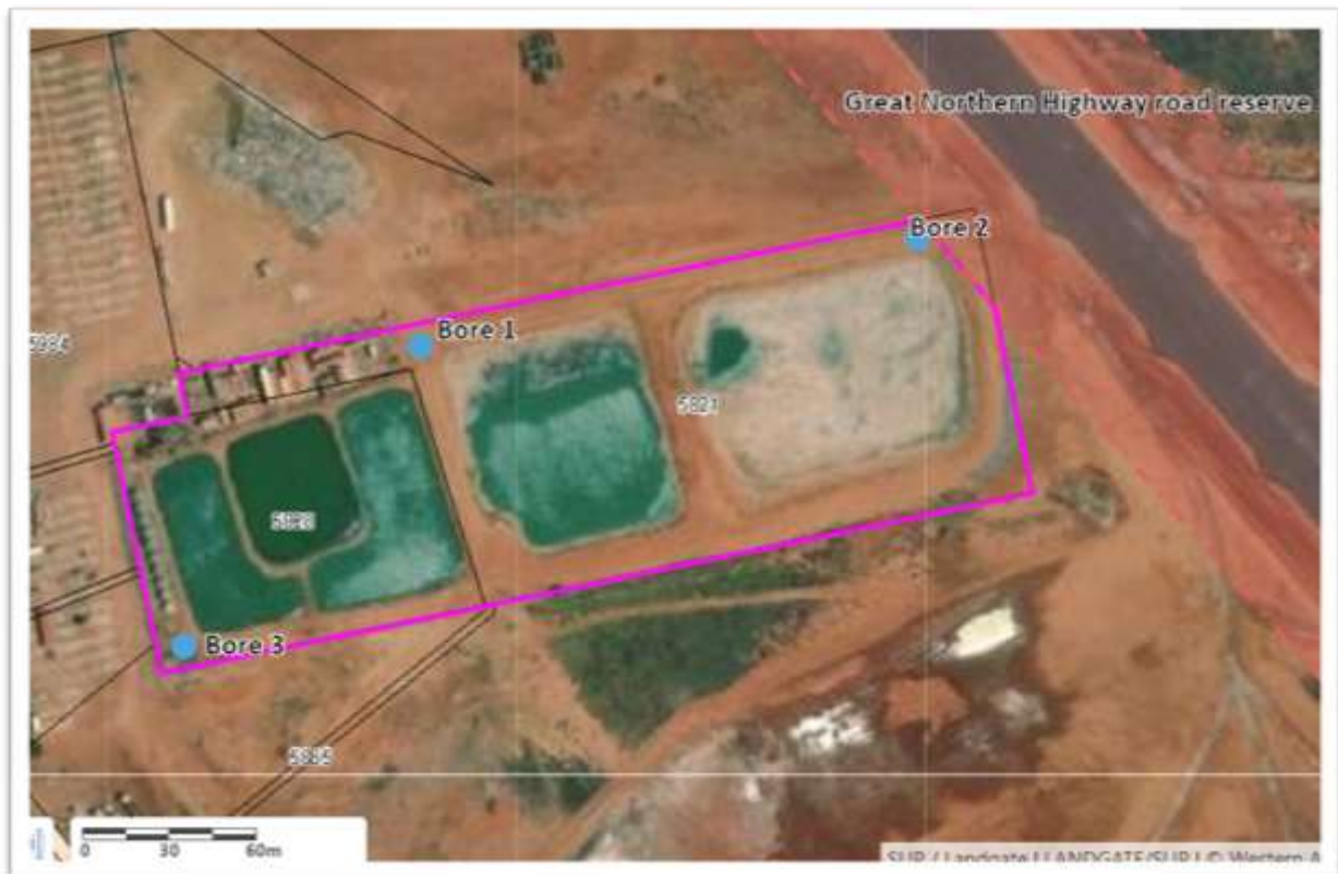
Figure 5: Applicant's proposed groundwater monitoring network
