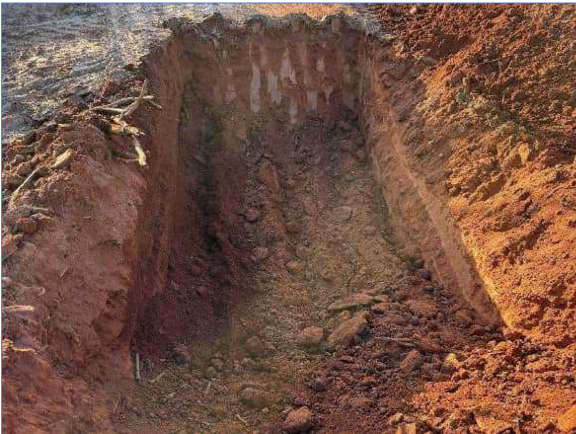
Plate 86: TSF-TP19 – Excavation to refusal
