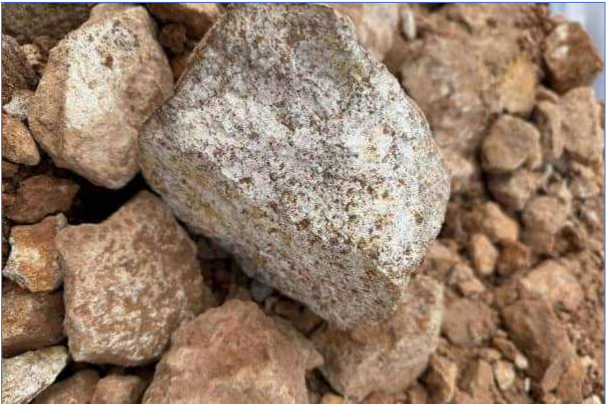
Plate 6: TSF-TP-01 - Granite rock HW/DW
