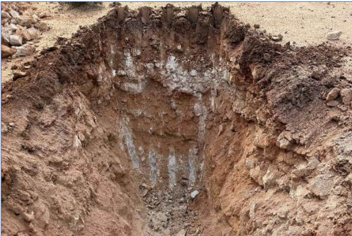
Plate 2: TSF-TP-01 – Excavated to refusal
