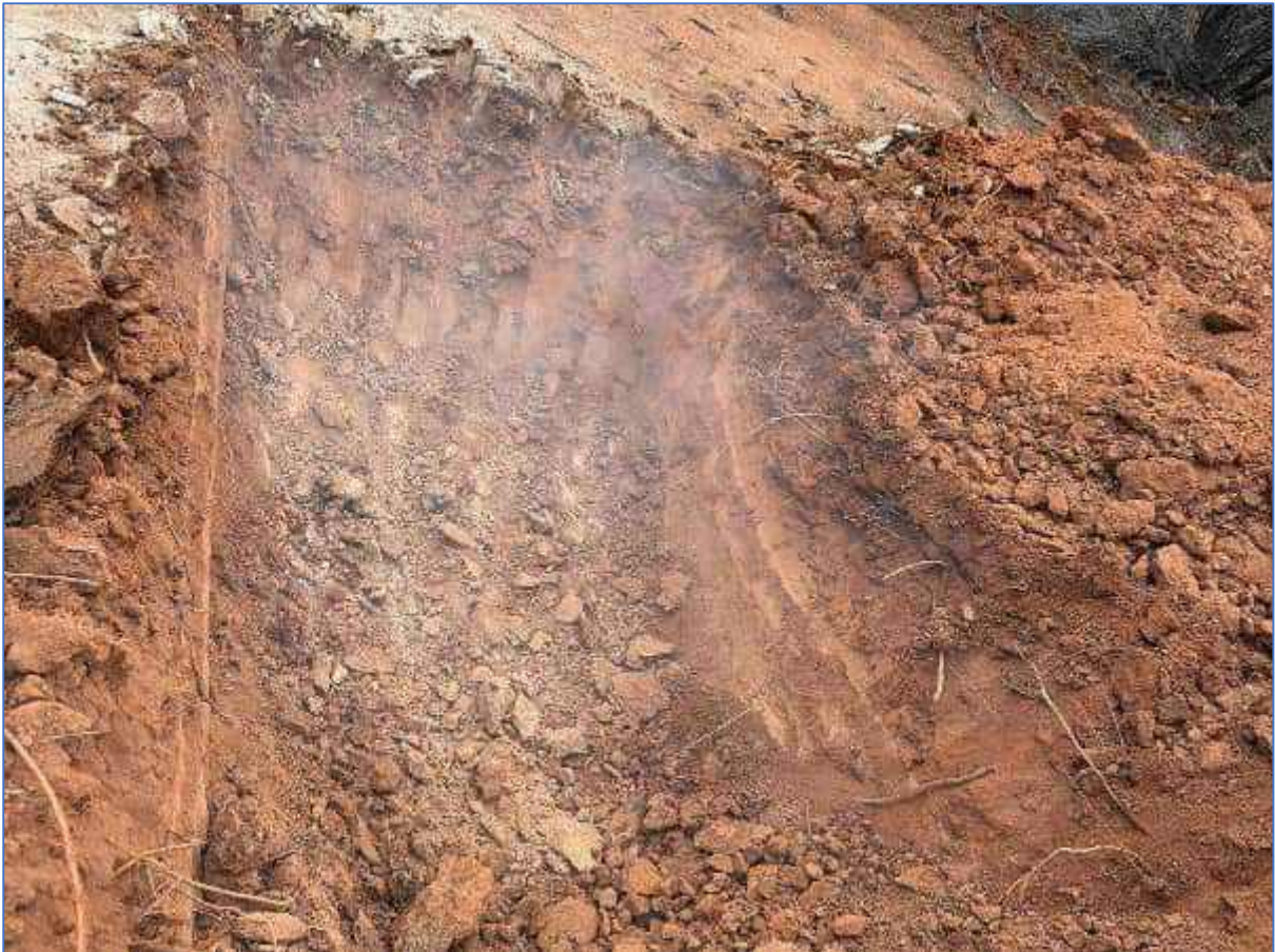
Plate 32: TSF-TP07 – Excavation to refusal
