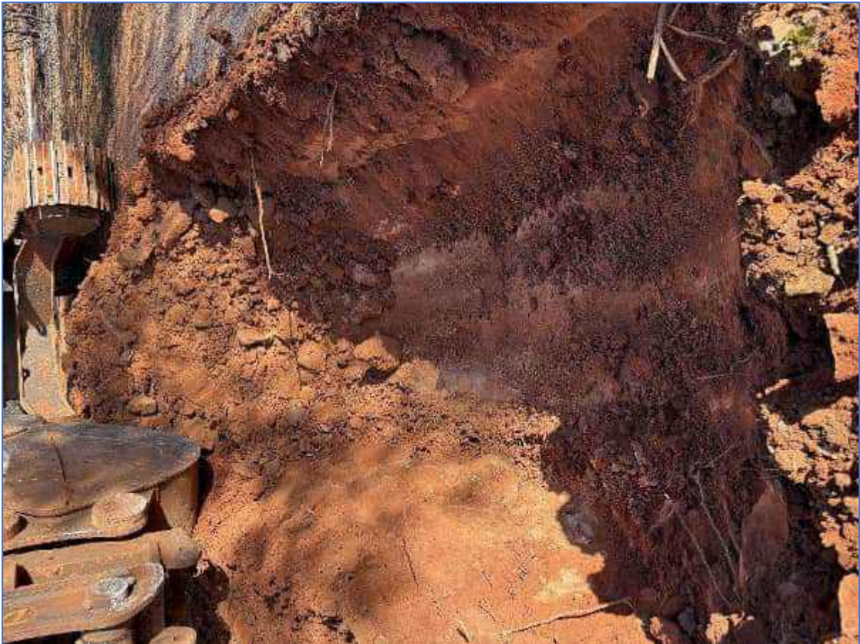
Plate 62: TSF-TP13 – Excavation to refusal
