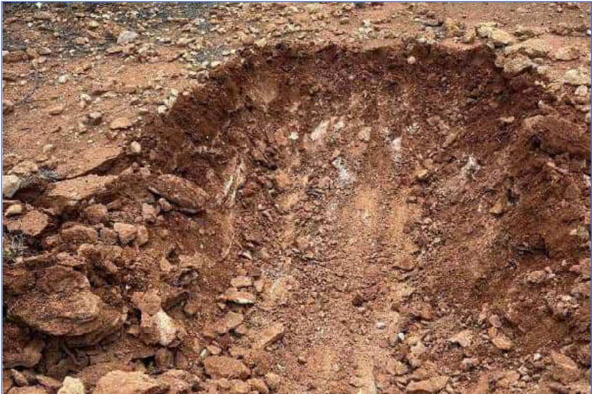
Plate 8: TSF-TP-02 – Excavation to refusal
