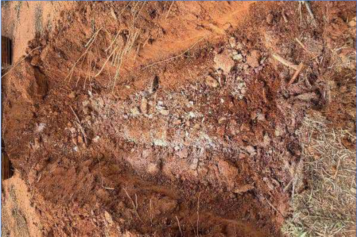
Plate 37: TSF-TP08 – Excavation to refusal
