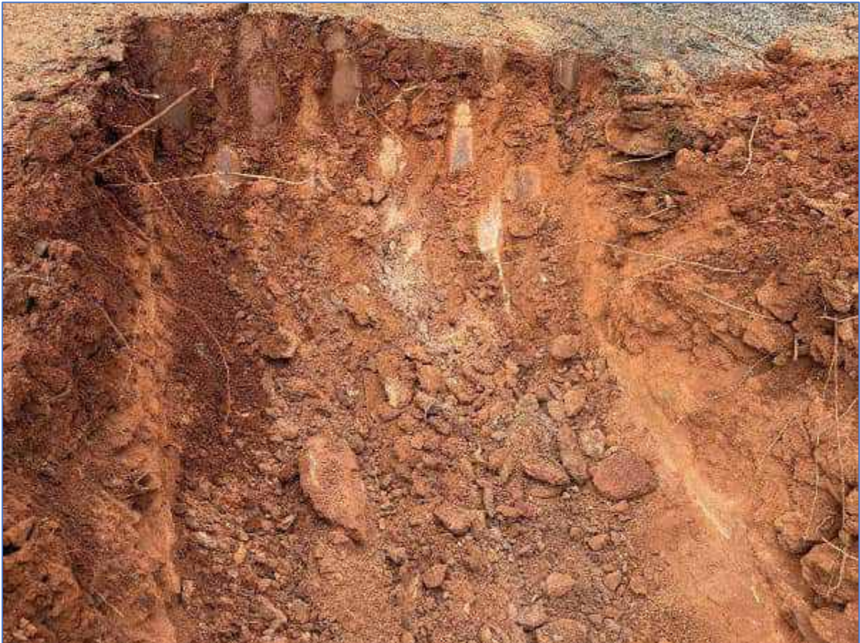
Plate 24: TSF-TP05 – Excavation to refusal
