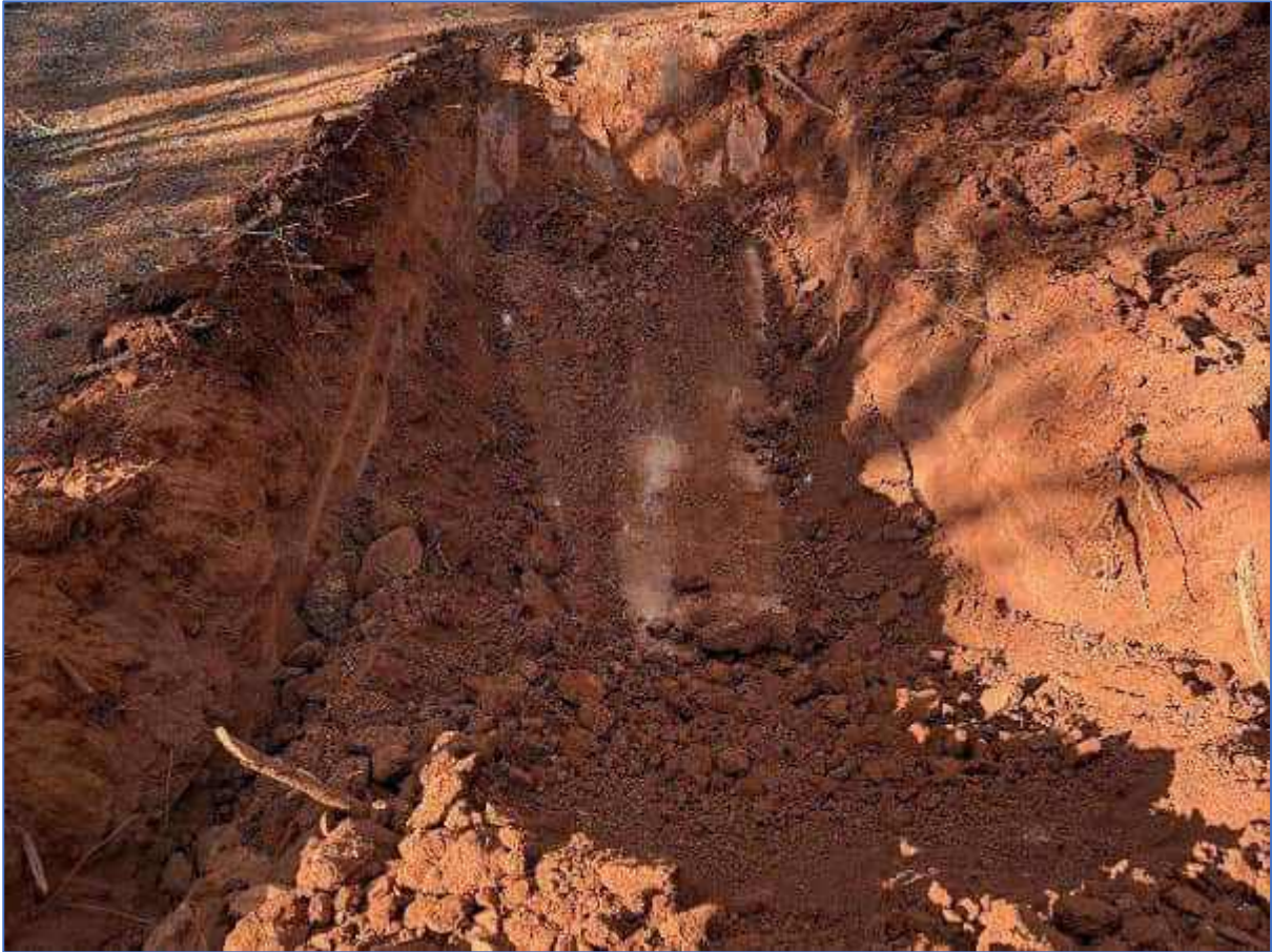
Plate 65: TSF-TP14 – Excavation to refusal
