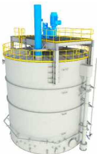
Figure 5-2 – Oxidative Leach Reactor
