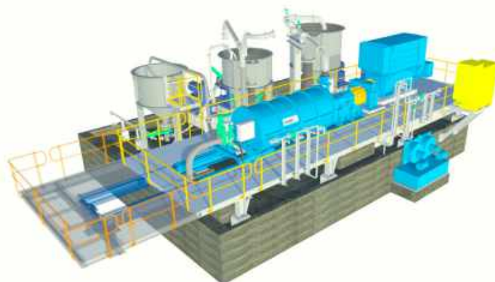
Figure 5-1 – IsaMill™ Grinding Plant
