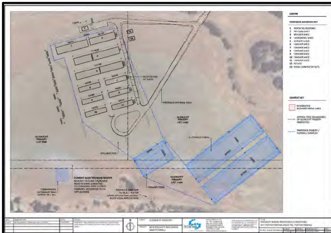
Figure 18 Proposed siting and dimensions of treatment and storage ponds
