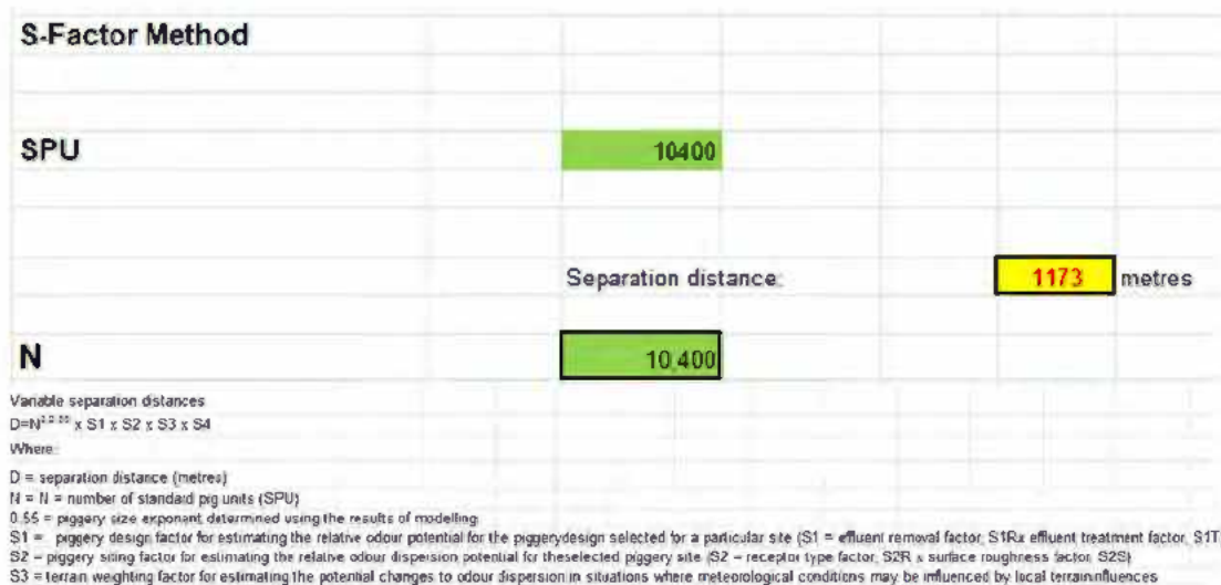
Figure 22 S-Factor separation distance outputs from APL, 2025.
