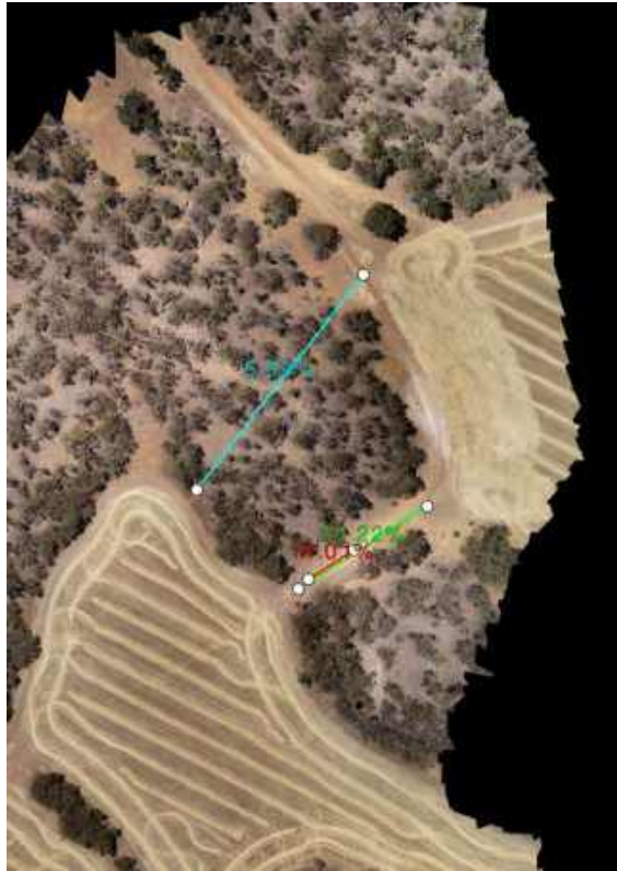
Figure 16: RTK survey gradient map showing slopes of the proposed alignment and southern clearing
