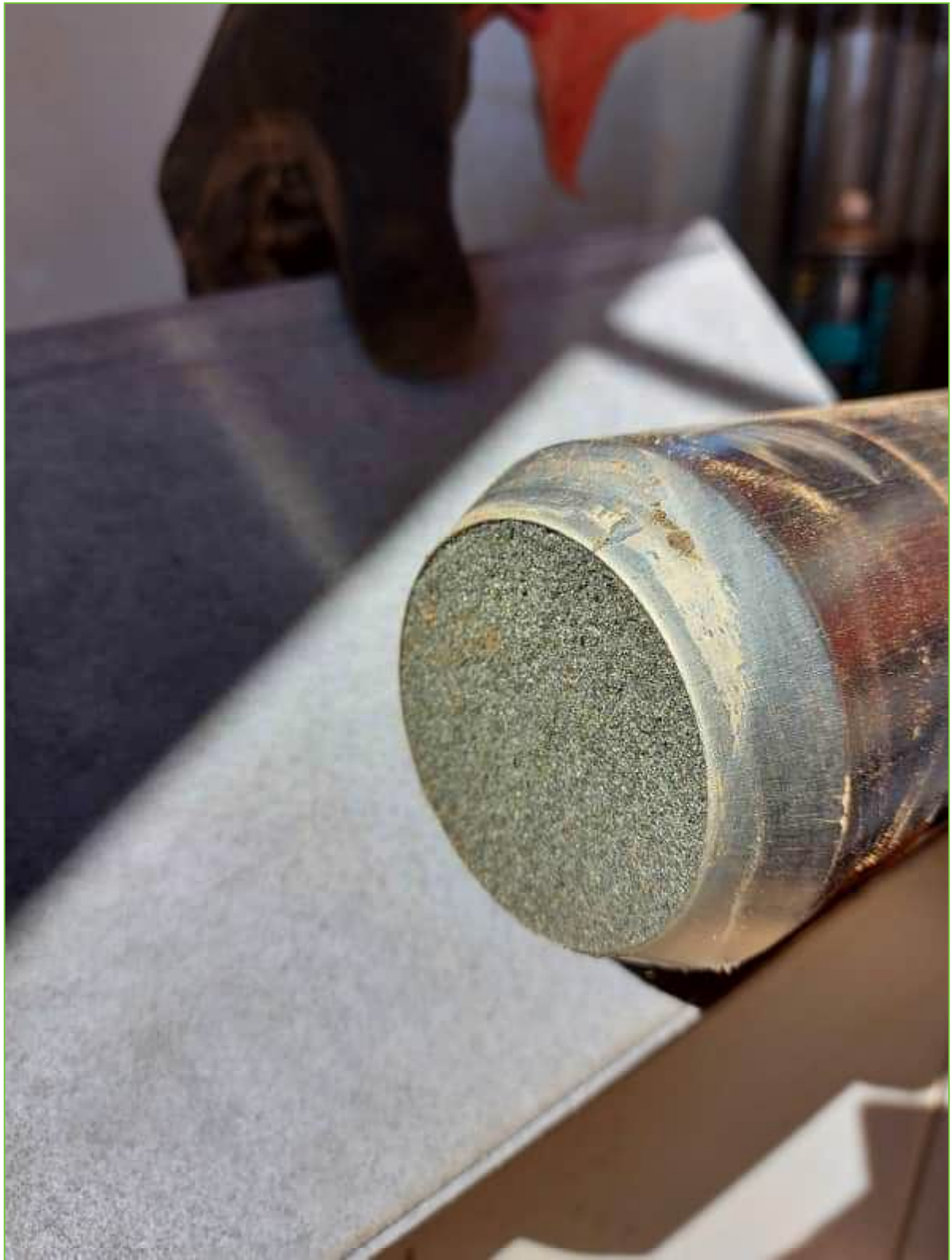
Figure 3-2 Push tube sampler end with extracted undisturbed in-situ Coarse Tailings material
