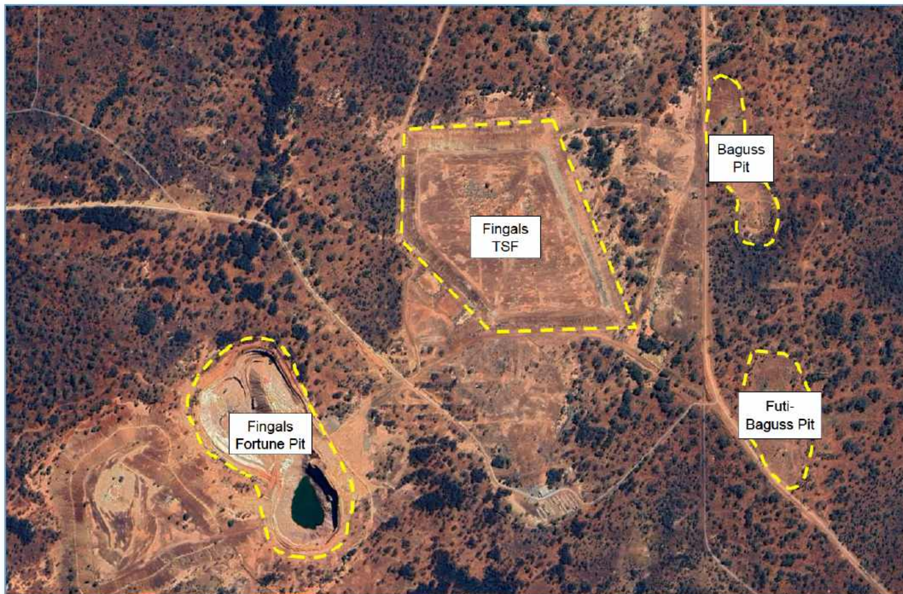
Figure 1-1: General arrangement of Fingals TSF and surrounding open mine pits in-filled with tailings
