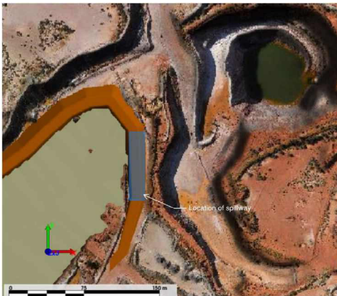
Figure 7.6 Donut Beta TSF spillway location
