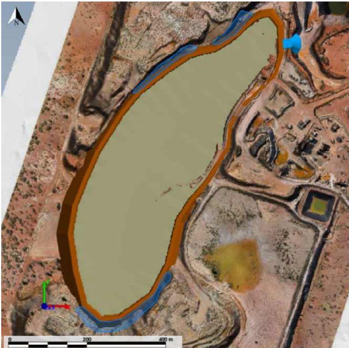
Figure 7.44 Potential areas of isolated ponding along the Donut Beta TSF and waste dumps
