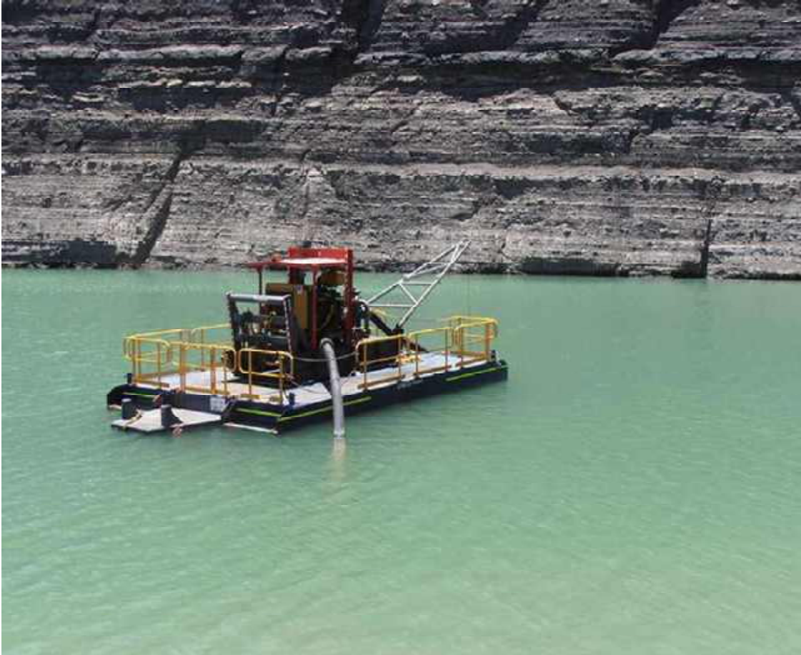
Figure 5.3 Photo of a typical pontoon decant system
