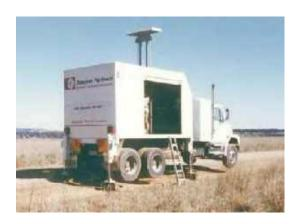
Figure 2: Purpose built CPT rig
