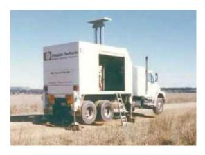
Figure 2: Purpose built CPT rig
