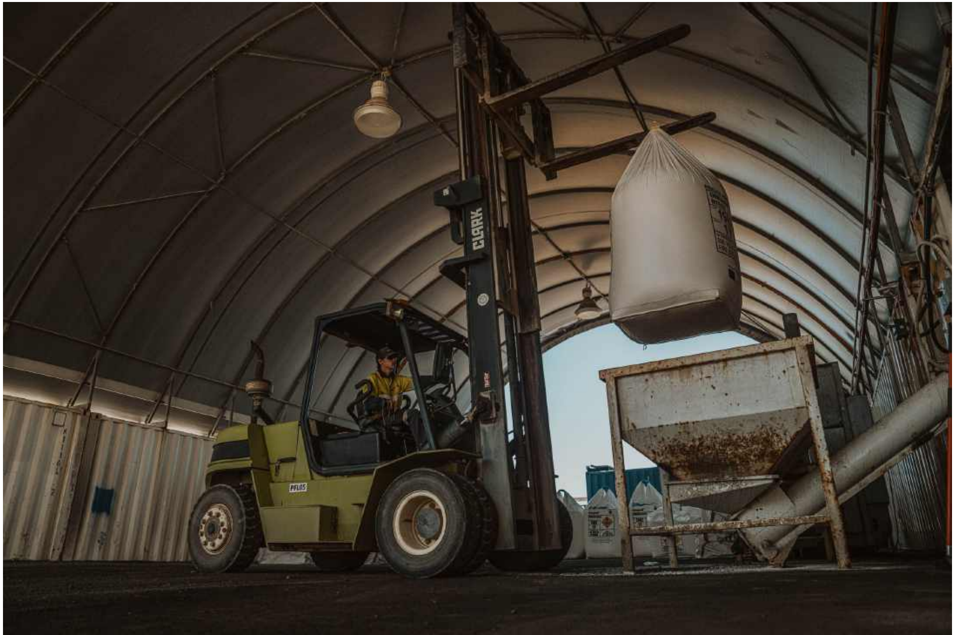
Figure 3 AN being debagged into a hopper where it is augered into the ANE plant
