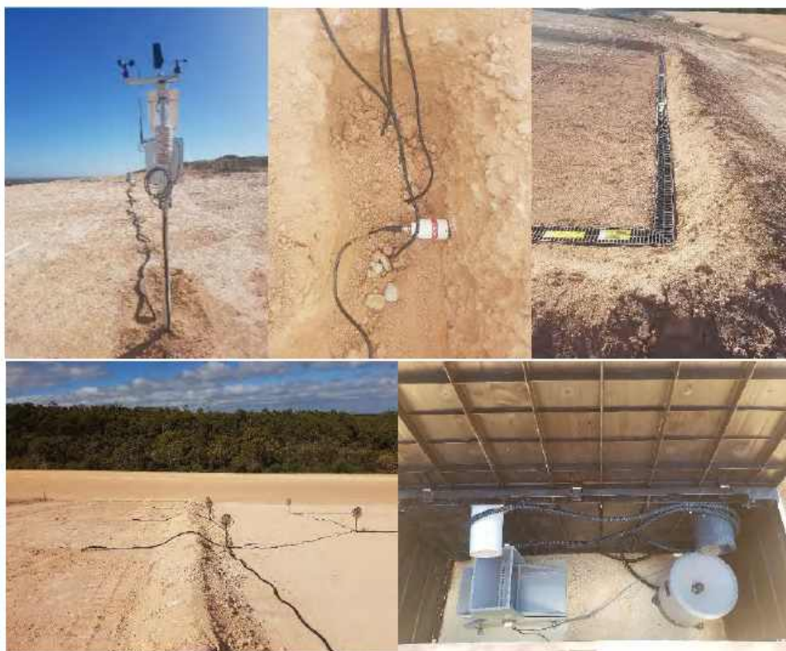
Figure 1 Installation Photos showing Weather Station (top left), SM150T sensor installed at 0.4 m depth (top centre), runoff collection gutter (top right), location of sensors with lysimeter to the left (bottom left), downslope installation of runoff (left) and drainage (right) gauges (bottom right)
