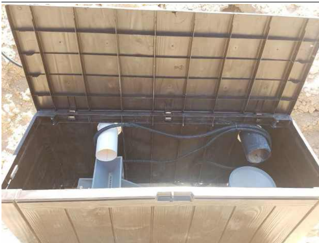
Plate 8 Runoff gauge (left) and drainage gauge (right) installed in storage tub downslope of lysimeter
