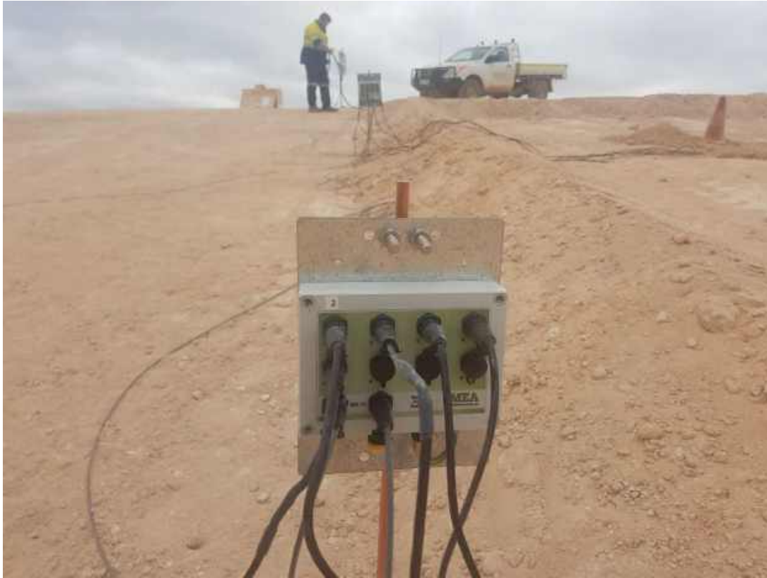
Plate 5 Field Station 2. Channels 1-5 contain moisture sensors with Channel 1 with shallowest sensor and Channel 5 deepest sensor
