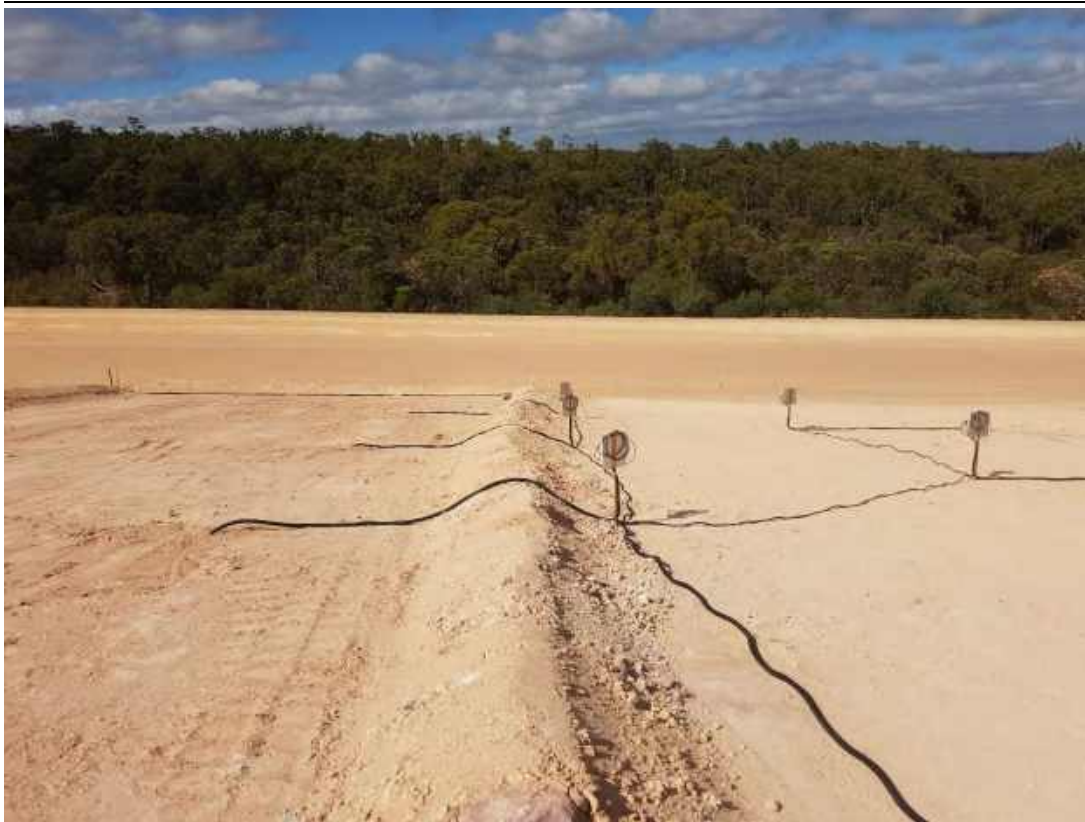
Plate 4 Proposed Photo Point 2. Standing at north-western corner of lysimeter. Five field station locations and conduit to monitoring nests shown
