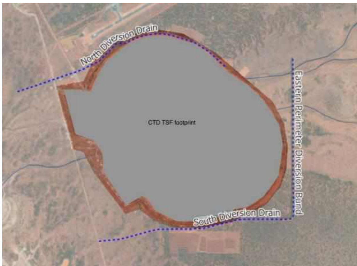
Figure 11: Surface Water Management Infrastructure CTD TSF
