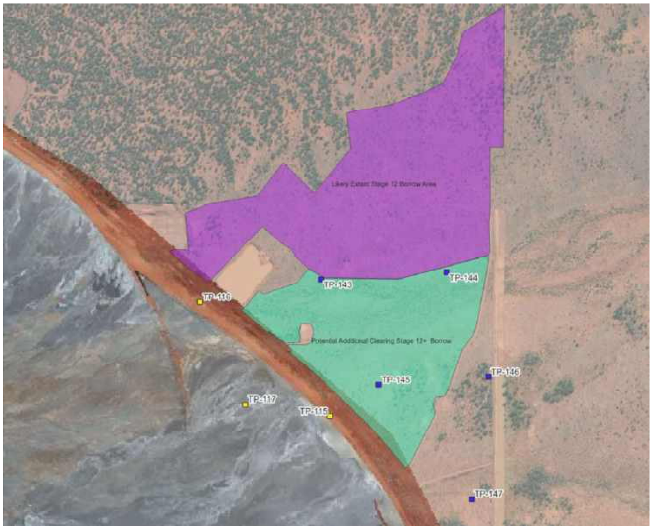
Figure 5.3 Nominated borrow area clearing extents for stage 12 raise construction
