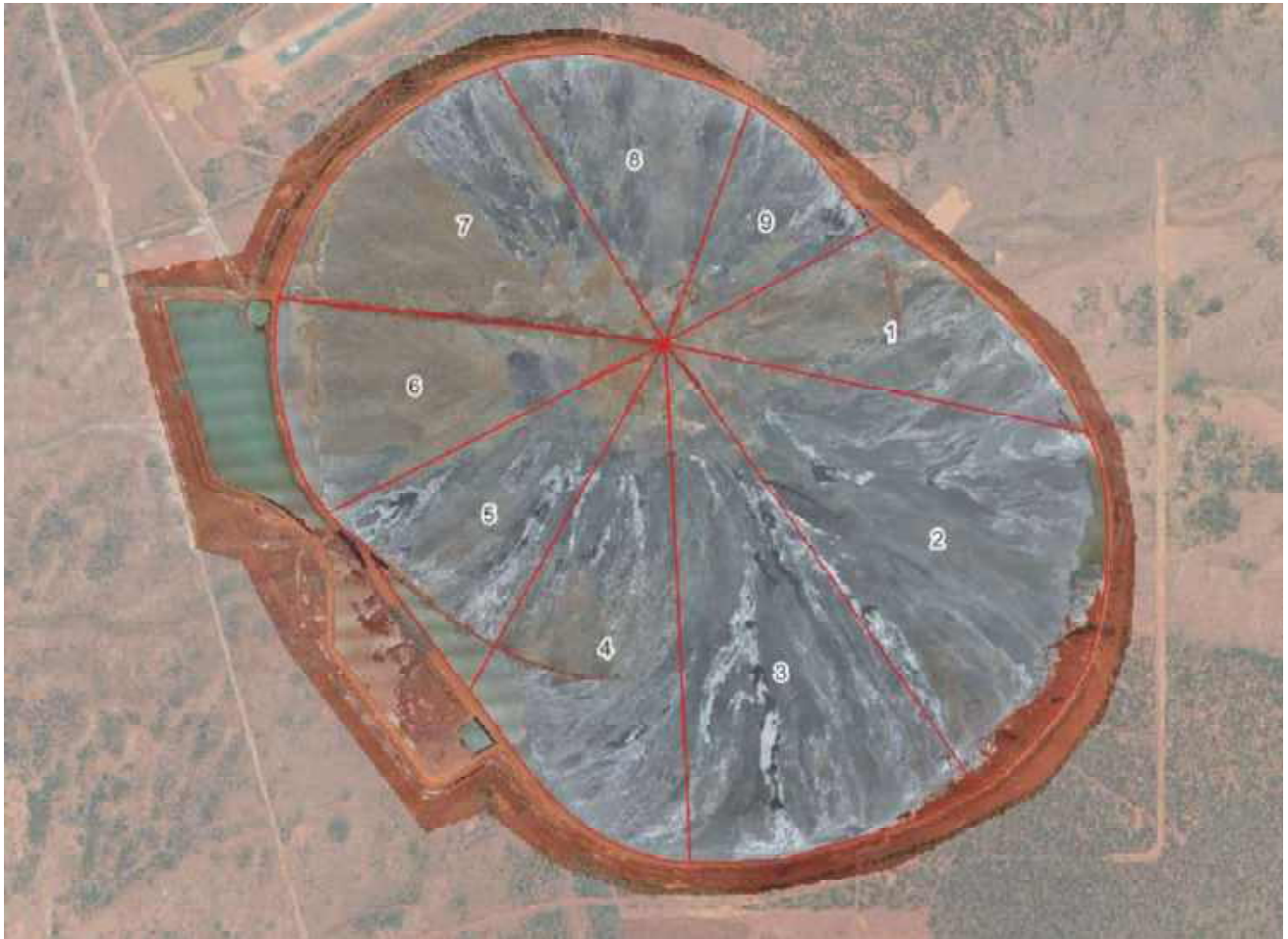
Figure 8.1 CTD TSF deposition sectors
