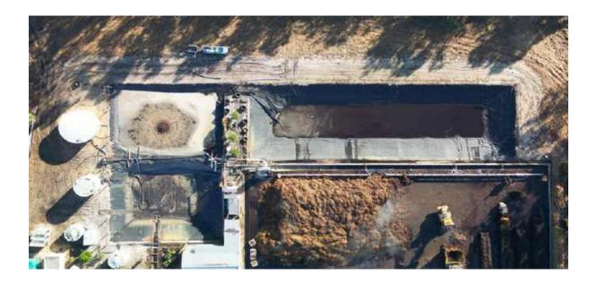
Dam 1, will be used to contain all run off leachate from daily operations for the duration of maintenance and replacement of dam liners (14 days)
