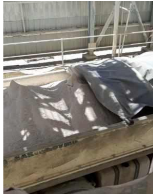
Figure 5: LKD prilled product being sealed in tipper truck for transport
