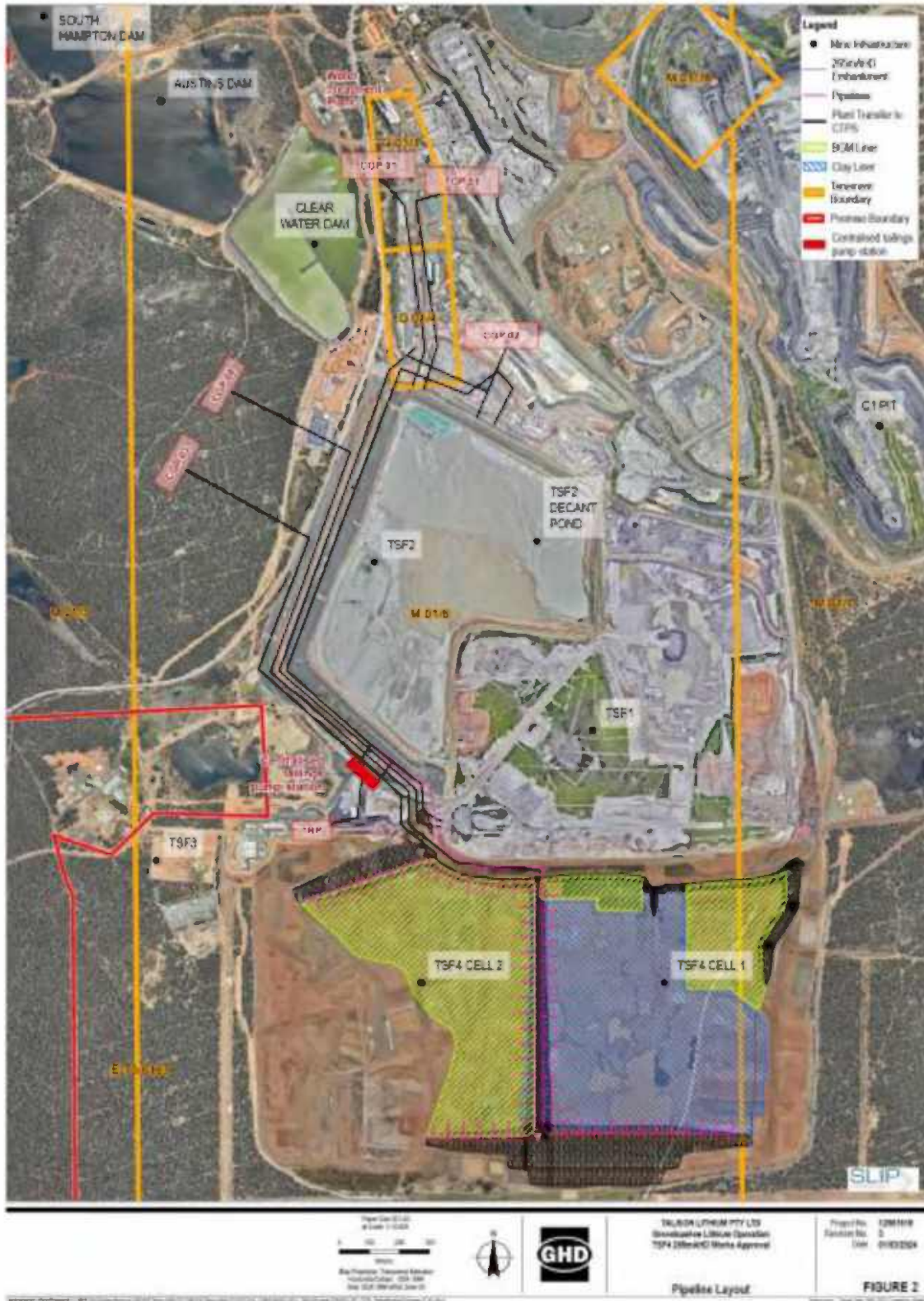
Figure 20: Tailings pipeline discharge into TSF4 and decant return pipeline
