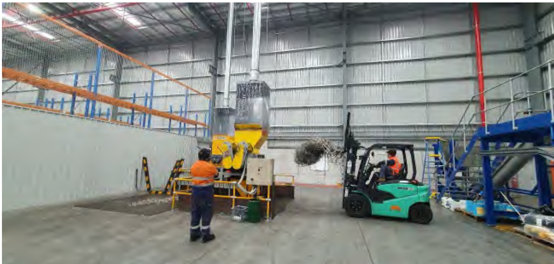
Figure 5: Metal turnings shredder and forklift
