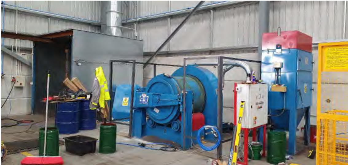
Figure 6: Plasma cutting (left) and shot blasting (centre, right) equipment
